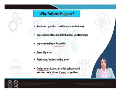
And whatever is the case, whether it is a full failure or partial failure, we need to understand that why failures typically happen and then several reasons for failure to happen. The most common are these. Such as there are some service or operation condition changes, which could be due to not proper using that are due to the misusing of the service or the operating conditions or this could be also because of the improper maintenance.
