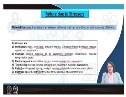
Now, failures often happen due to the stressors now, what is the stressor? This material stressor are actually the external influence that can be direct or indirect cause for the failure. Now, there are six different kinds of stressors that are typically present and that may have an influence on the failure. There could be mechanical stresses, and this mechanical stresses include static or the cyclic load like whether it is a monotonic condition or fatigue condition that is being applied.
