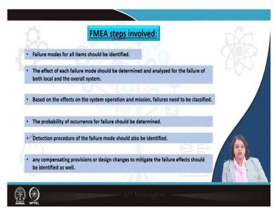
So, if we are talking about the steps here for FMEA we know that for this to be used, actually failure modes of all items should be identified at the very first place. So, how the each of these components are being failed, that needs to be understood and the effect of each failure mode should be determined and analyze for the failure of both the local performance as well as the overall system.
