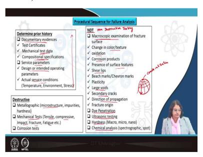
So, let us see the procedural sequence that are used for the failure analysis. So, first of all, we need to find out the prior history and for the prior history, we typically have to rely on that documentary evidences. So, there are the test certificate, some mechanical test data the compositional specifications that has been already provided by the supplier or vendor or the manufacturer.
