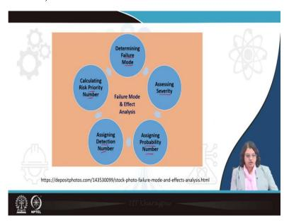
So again when we are looking for the different steps in a flowchart, we see that we initially need to understand the failure mode. And based on the severity of the failure mode for each of the component, we assign a probability number so that we can understand that, this has a possibilities of failure may be a higher possibilities of failure or lower possibilities of failure
