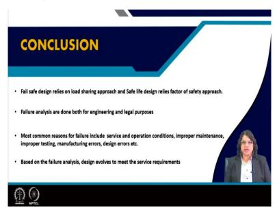
So, let us conclude this lecture with the following points here that Fail Safe design particularly relies on load sharing approach and on the other hand Safe Life design as we have seen relies on the factor of safety and that ensures that no failure within a certain time period. Failure analysis are done both for engineering purpose as well as for legal purpose and we have seen that how legal purpose could actually lead to a very important factor for pursuing the failure analysis.
