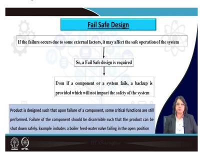
Now, if the Safe Life design is not appropriate, we have to go for the Fail Safe design. So, let us see what is that? Now, if the failure occurs due to some external factors, it may affect the safe operation of any of the component in this case, we are talking about an aircraft, but this is true, this is valid for any of the component and for that, we need a Fail Safe design.
