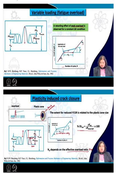
So let us talk about variable amplitude loading, particularly when we are having an overload just one cycle of overload. So what we are seeing here is that there is a regular fatigue cycle that has been applied with particular values of  $\Delta K$  at every cycle and then suddenly there is an overload and once the overload is gone then again it is resuming back to the previous cyclic mode with the same values and all.
