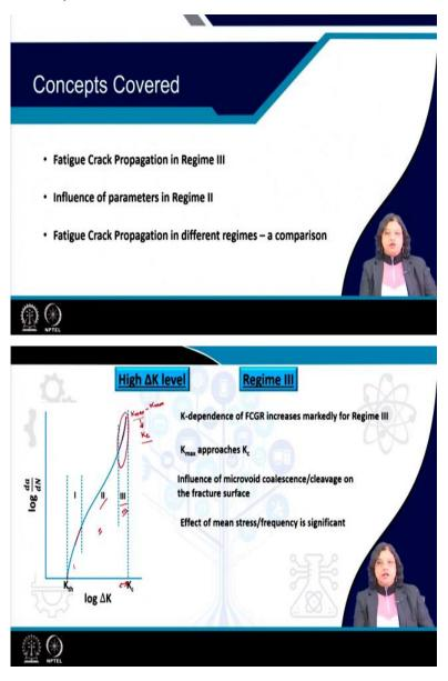
Particularly we will cover the topic on the fatigue crack propagation in regime III that means the high  $\Delta K$  regime and then we will be also talking a bit on the influence of the parameters in regime II which essentially controls the main fatigue crack growth rate part, and
