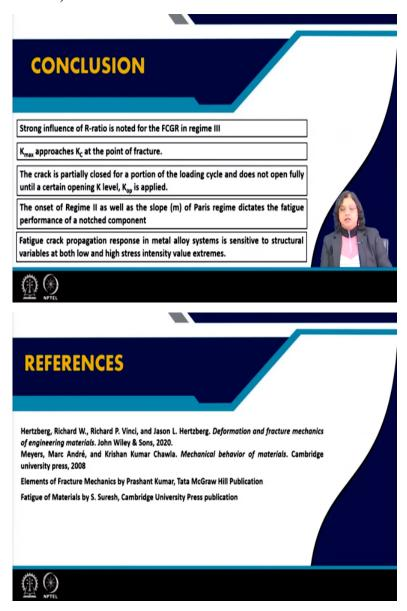
So with this let us conclude this lecture with the following points that strong influence of R-ratio is noted for the fatigue crack growth rate curve, particularly in regime III and  $K_{max}$  approaches the critical value of K at the point of fracture and that is the terminal point of the da/dN versus  $\Delta K$  curve.
