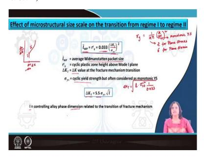
And if we are looking into the microstructure aspect it has been found particularly initially studied for steel and it has been found that a particular relation is being followed based on the microstructure size as well as the  $\Delta K$  value for this transition.
