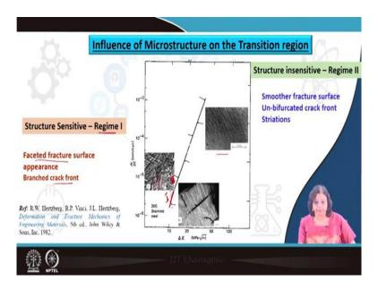
To see that, to understand that actually, we need to look into this da/dN and versus  $\Delta K$  curve more precisely and particularly, the transition between this regime I and regime II is what is significant. So, this one here shows just the onset of regime II and that means that the small part here is actually regime I. So, there is a different mechanism completely different mechanism is being followed for regime I and II and this transition is happening over this particular location.
