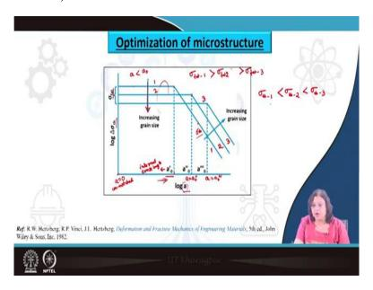
And that means that we need to have an optimization of the microstructure. So, in one case, we are seeing that so, this is graph for log of  $\sigma_{th}$  or the threshold stress range versus a or the crack length, at this point at the origin we know that a is 0 here and that means that this is basically an un-notched component, for the case of un-notched component fatigue strength is what we are getting here, here  $\sigma_{fat}$ .
