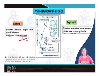
So, let us now once again go back to the concept when we found a relation between the plastic zone size as well as a Widmanstatten packet size versus the  $\Delta K_T$ . So, what is being shown here once again is the da/dN versus  $\Delta K$  curve.
