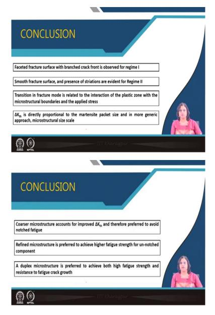
So, let us conclude this lecture with the following points here that we have seen that faceted fracture surface with branched crack front are observed for regime I. And on the other hand, for the case of regime II smooth fracture surface and presence of striations are noted and the transition is actually related to the interaction of the plastic zone and the microstructural boundaries.
