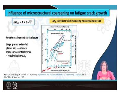
So, that has a pretty much influence on the fatigue crack growth certainly. So, that means that we can aim to achieve higher and higher microstructural size so, that we can increase the value of  $\Delta K_{th}$  and our purpose for the regime I have the higher value of  $\Delta K_{th}$  such that the onset of the growth of the crack can be delayed.
