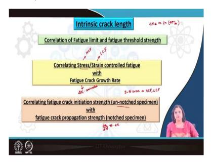
So, far we have seen how the external parameters can be controlled to get the value of the  $\Delta K_{th}$  or the threshold value for the onset of the crack growth and let us see how physically this can be related to the other kind of fatigue that we have talked so far.
