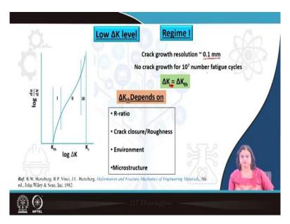
So, to begin with, we have already introduced the concept of  $\Delta K_{th}$  or that is the threshold stress intensity factor range that is required for the onset of the growth of the crack. So, even if a crack is existing in a material, we need a certain value of  $\Delta K$  to be applied such that the crack can start growing. So, let us say we use some instrument to resolve the crack and let us say the resolution of that instrument is 0.1 mm.
