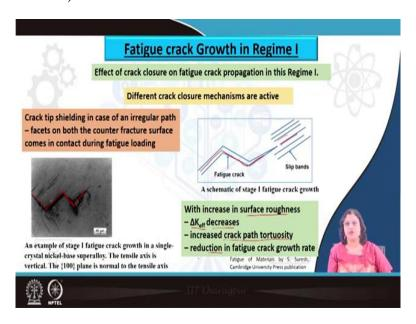
Now, let us see how the effect of crack closure is active for the case of Regime 1, actually what happens here is because of the torturous nature of the crack path, often we see that there is a crack branching or there is a deviation in the crack growth direction and that is one of the way by which the crack closing activity is valid for this Regime 1, there are other different crack closure mechanisms are active and particularly we have the crack tip shielding effect.
