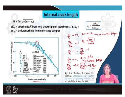
So, this intrinsic crack length has been defined so, far and now, we also needed to look into the practical significance of this and this can be only validated through some experimental results, which has been shown here for different kinds of materials such as different varieties of steel as well as non-ferrous materials such as copper and aluminium these are studied by different groups of scientists all across the world to get the different values.
