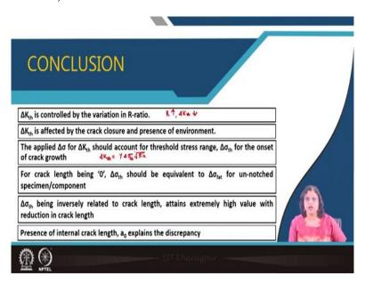
So, let us conclude this lecture with the following points that the  $\Delta K_{th}$  or the threshold value of the stress intensity factor range is controlled by several factors the prime one being R-ratio or the ratio of the minimum value of K by the maximum value of K and we have seen that an inverse relation is being followed, which means that R increases and  $\Delta K_{th}$  decreases.
