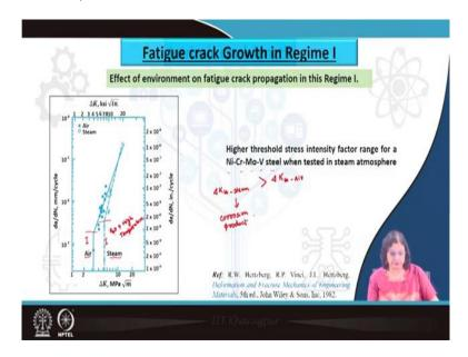
So, that was one of the factors, the other thing that is of interest here is the effect of environment. Now, environment we have seen earlier also that how fatigue could be influenced by the different environment or different atmosphere for that matter. So, here for example, we will show one experimental results for the failure of steel in different environment, one is in air and the other is in steam.
