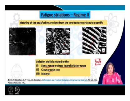
So, this fatigue striations now, if we look into this, you will see the first one image here shows that there is a micron marker of 5 micrometres this red colour here is 5 micrometres, and you can understand that this striation with are very, very small. In comparison, we have another one here, where same almost same kind of micro marker level is there, which is 4 micrometres.
