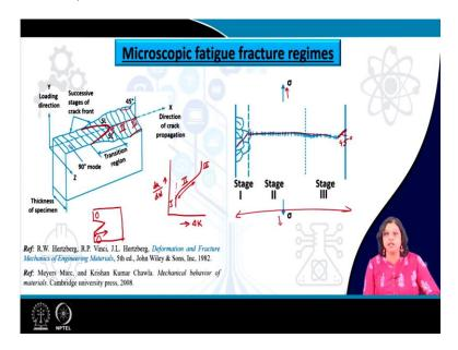
So, let us see what are the different regimes that we have already seen in the da/dN versus  $\Delta K$  curve, which looks something like this, we have the crack growth rate on the y-axis and we have  $\Delta K$  on the x-axis both this y and x-axis are in the logarithmic scale and we can see that this curve can be divided into 3 regimes.
