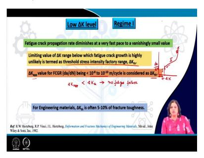
So, let us move on to the very first regime, which is the regime I, also known as the low  $\Delta K$  level, because this is the starting point for the FCGR curve, but we are coming here later, because the we were initially talking about the part which was the most significant in fatigue crack growth behaviour.
