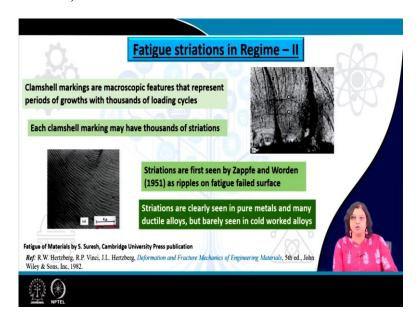
Now, further if we are looking just the fracture surface with the very low magnification microscope 1, then we can see the clamshell markings. So, these are the macroscopic features and just by looking on those kinds of features like clamshell markings or beach marks, or ratchets, which looks like steps, we can figure out that the component has undergone repeated loading, and actually, if we are considering even at a higher depth of focus.
