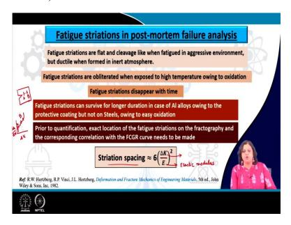
And particularly striation width is very, very important and not only the width, but other features of striations are very, very important for the Post-mortem failure analysis. So, let us see how it can be useful. Basically fatigue striations are the shape of this striations are very important to understand in case it is a flat one like a cleavage one, that actually signifies that fatigue has happened in presence of aggressive environment.
