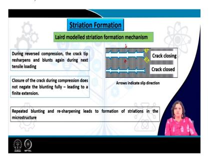
Now, this is one side like when we are applying the tensile stresses and furthermore, when we are applying the compression, the reverse compression stages, then the crack tip resharpens and then again it gets bland during the following tensile loading mode. So, this keeps on happening on every cycle. So, once it gets bland and then it gets a closed and then it gets resharpen again and again and for each of the steps actually each striations are forming.
