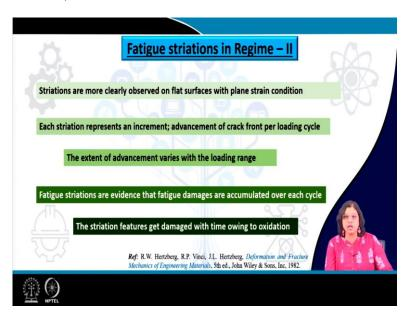
So, striations are particularly observed in case there is a flat surface and when the plane strain condition has been applied, as I mentioned, like regime II is the one where the crack growth is following 90° to the loading condition which is nothing but a plane strain condition being followed in such case only striations will be visible.
