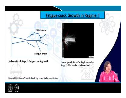
And that is particularly related to the growth of the crack in this regime which is affected by the slip bands present in the particularly in the ductile kind of material. So, you can see here, the left one is a schematic one and the right one is the actual image where you can see that this is the machined notch part here and how the crack is growing. And then there are the sleep bands and there are two opposite directions very well distinctly visible here.
