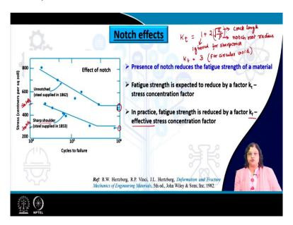
We have seen this earlier also while we were discussing about the SN curve that is the stress amplitude versus number of cycles to failure curve, we have seen that in presence of notch that is for a north specimen this SN curve is quite below the typical SN curve of an unnotched specimen.
