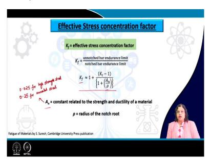
So, the  $k_f$  is actually given by the ratio of the unnotched bar endurance limit or fatigue strength divided by the notched bar endurance limit. So, that dictates the value of  $k_f$  in a more generalized form we can express  $k_f$  by this relation here. So,  $k_f$  is given by  $1 + \frac{k_t - 1}{1 + (\frac{A_n}{\rho})}$ . Once again, we are introducing another parameter here which is  $A_n$  that is a constant related to the strength and ductility of a material.
