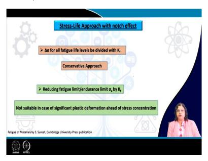
Now not only that, if there is this notch effect already active, we should also think about how the stress life can be determined the fatigue strength or the fatigue life can be determined in presence of a notch already existing. So, either there are two ways to do that either we can divide the entire  $\Delta \sigma$  or the stress range that has been applied by  $k_f$  for the effective stress concentration factor but this approach will be too conservative.
