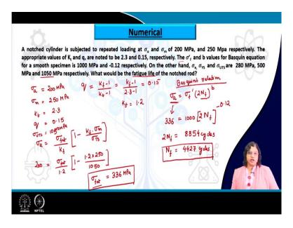
So, this could be better understood, how this understanding can be related to the fatigue strength as well as the fatigue life of the specimen that can be appreciated based on this numerical. So, what it says here is that there is a cylinder which has a notch in it and that is subjected to repeated loading all the parameters of loadings are given here as  $\sigma_a$ .
