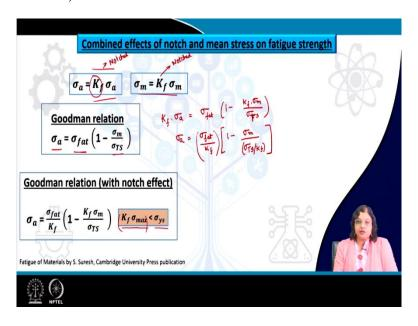
Now, this is interesting to note also that in presence of the notch, now we have seen earlier that if we are varying the mean stress of the mid of the cyclic loading then the fatigue performance is varying completely. We have seen this on the basis of the Goodman diagram and Soderberg relation as well as this Gerber relation etcetera. So, let us see how does it affect in in case of a notch present in a so called smooth bar now.
