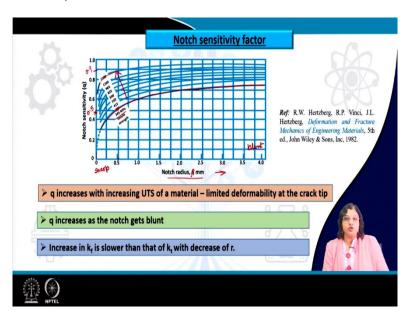
So, here is a graph showing the experimental results, for varying the notch sensitivity with the notch root radius. This is typically explaining the q versus  $\rho$  curve and what we are seeing here is that for each particular strength value if we are talking about the tensile strength of the material each graph actually signifies the tensile strength remaining constant. So, in this case the first one is 345 MPa.
