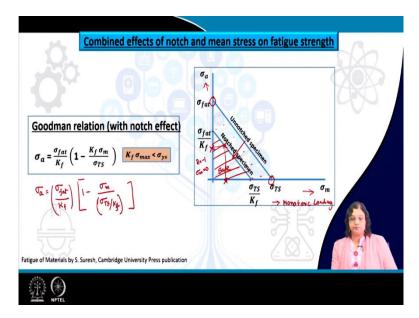
And this is actually determined or this is once again plotted based on the  $\sigma_a$  versus  $\sigma_m$  curve we have explained this earlier also that sigma m is the mean stress and at this point the x axis which means that  $\sigma_a$  is 0. So, basically this means the monotonic loading, so similar to tensile testing. And for that case fracture occurs at the point of ultimate tensile strength of the material.
