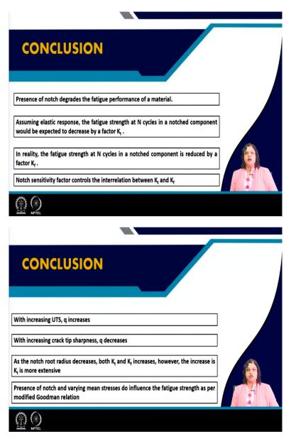
So, let us conclude this lecture with the following points that what we have seen here, is presence of notch certainly degrades the fatigue performance of a material, and considering the elastic response, the fatigue strength at n cycles in a notch component would decrease by a factor  $k_t$ . But this is not happening in practice rather the fatigue strength is reduced by a factor  $k_f$  or the effective stress concentration factor.
