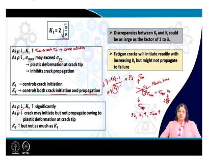
So, what we have seen or what we know so far is that  $k_t$  is typically given by  $2\sqrt{\frac{a}{\rho}}$  for a sharp crack. So, let us see if there is a sharp crack like this on which we are applying stress  $\sigma$  or  $\sigma_a$  for example then at the tip of the notch we are getting  $\sigma_{max}$ . Because of the stress concentration and  $\sigma_{max}$  is nothing but  $\sigma_a$  multiplied by the stress concentration factor and this is nothing but  $2\sqrt{\frac{a}{\rho}}$ .
