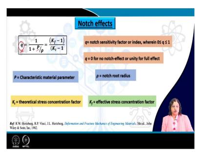
So, typically this is related to another parameter here which is known as notch sensitivity factor. How much the notch is affecting the fatigue behavior of the material that is reflected through this parameter q. Typically the value of q lies within 0 and 1. When it is 0 that means that there is no notch effect or there could be no notch at all. And the value of q could be 1 or unity in case there is a complete notch effect is active.
