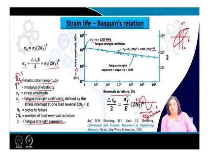
So, for that we also need to find out the relation between strain amplitude and the number of cycles. So, that is given by Basquin's relation particularly for the elastic part. So, as we have seen that elastic strain so within the elastic limit or below the yield point of the material yield strength of the material it is the stress amplitude that is of most significance and the strain life based on the elastic strain amplitude is determined based on the stress amplitude itself.
