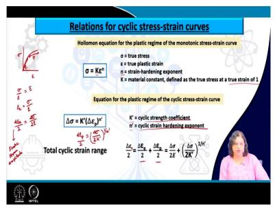
So, then let us look into the relation between the stress strain curve. So, what are the different kind of relation. First of all, if we are talking about the stress strain curve, it has two segments like the elastic part and the plastic part. So, let us say we have a stress strain curve like this whether it is monotonic or cyclic whenever we have a stress strain curve we have some part which is the elastic part and then the other part which is the plastic part.
