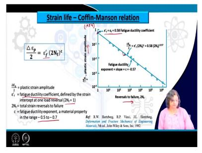
So, next we should move on to the plastic part and let us see that how that is relevant to the number of cycles for failure. So, that has been this kind of relation for the plastic strain amplitude has been found independently by Coffin and Manson both at the same year of 1954 and the relation is again given by the strain plastic strain amplitude equals to  $\varepsilon'_f (2N_f)^c$ .
