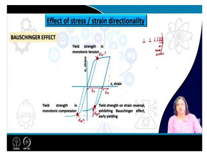
So let us begin with the Bauschinger Effect and the role of Stacking Fault Energy as the very first instance. So, what we have seen in the previous lecture is that when we are applying cyclic loading in the strain control mode there could be hardening or softening of the material just because of the cyclic loading or the repeated loading and this can be reflected in terms of the Bauschinger Effect.
