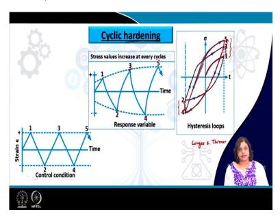
Now, let us see how this is reflected in the hysteresis loop also. So as I mentioned for the strain controlled one this is the stress output in this case for the case of cyclic hardening, the stress is increasing at every cycle so we are talking about three cycles here 1, 3 and 5. So 1, 2, 3, 4, 5 and we can see that the stress values in both the positive and the negative directions are higher from the the previous values and that is nothing but a cyclic hardening.
