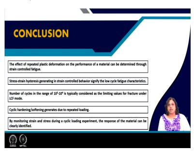
So in conclusion what we have discussed in this lecture is the following, the effect of repeated plastic deformation on the performance of a material can be determined through strain control fatigue and basically what we are generating here from the strain control fatigue is the stress strain hysteresis, so instead of a straight line for the elastic loading now we have a hysteresis curve and that signify the low cycle fatigue characteristics.
