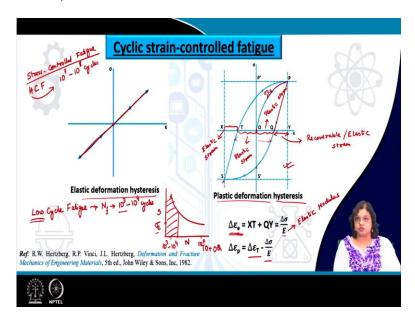
So when we are talking about cyclic loading or repeated loading so far while considering the stress control fatigue we have seen that the fatigue strength of a material can be achieved even at a stress amplitude value which could be lower than the yield strength of the material so that manner specimen is supposed to undergo only elastic deformation and there should not be any failure or any plastic deformation at all.
