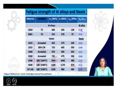
So, here are the results for some of the commonly used engineering materials particularly metallic systems. So, we have some aluminum alloys and based on the heat treatment condition, we see that there is some changes in the ultimate tensile strength UTS or  $\sigma_{TS}$  and that yield strength of the material. And that also leads to some change in the fatigue strength of the material.
