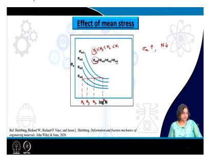
So, what we are seeing here is relation something like this, where the  $\sigma_a$  versus N plot similar to the SN curve and what we are seeing here is for the different values of  $\sigma_m$  which is the mean stress we can see the different SN curves for that the trend is still the same, but the position of the curves are different.
