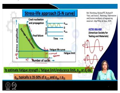
So, if such is the case, we have now also seen that how we can understand the fatigue performance of this through the SN curve, through the Wohler curve and which looks something like this. The y-axis shows the stress amplitude and the x-axis shows the number of cycles and we are getting a typical form of curve which looks something like this.
