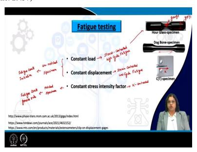
So, let us see that how we can test fatigue. Typically, there are different ways by which fatigue testing has been done. And we can do it in the following way. We can do it either in the constant load mode. So, basically what we do here is to control the stress. So, this is
