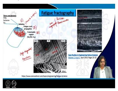
So, these are the micro structures or the fractographs. If we are looking into the structures of the fracture surface that is termed as the fractography. So, typical signatures of fatigue fracture can be seen from the fractographs. Particularly if we are looking on the whole component, fatigue typically has these three locations.
