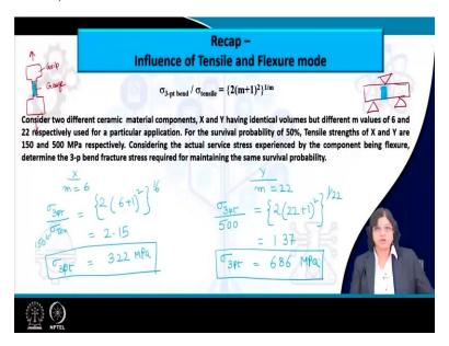
Ok, so, with this will move on to another problem that we have discussed in the last lecture, which is the difference in the fracture strength values if we are changing the mode of loading, right. So, for tensile or flexure mode of loading, we have seen that the flexure mode always gives us higher fracture strength in comparison to that for tensile loading.
