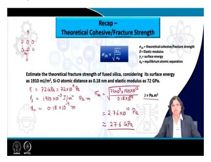
So, coming to the numerical part, in the last class, we have discussed about the theoretical strengths of material theoretical shear strength as well as theoretical cohesive or fracture strength of a material. So, what it essentially means is that, if we have atomic lattice like this applying stress over it at one point this is going to break and form new surfaces.
