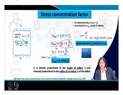
So, if we want to quantify that, this is how we do the  $\sigma_{max}$  at this point at the corner of the crack, at the tip of the crack or corner of any change in the component structure, we are going to get  $\sigma_{max}$  instead of  $\sigma_a$ . So,  $\sigma_a$  is what we are applying the stress. So, this could be  $\sigma_a$ , and what we are getting at the tip of the crack is nothing but  $\sigma_{max}$  and this is held by a relation as
