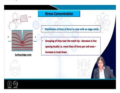
Ok, so, what happens, when there is a crack present in a component, this is what exactly happens, we are applying stress on both direction and these are the lines of force, we know it is very similar to the magnetic lines of force, the lines of force in case of a perfect component would be something like this.
