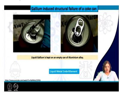
So, here is very practical example that I thought of demonstrating which shows how gallium will behave in presence of aluminum. So, liquid metal embrittlement concept for the combination of aluminum and gallium. Now, this is a coke cane made of aluminum we all know that these are the aluminum cans used for this kind of soft drinks and then here we see that piece of gallium in the liquid state is being put on this.
