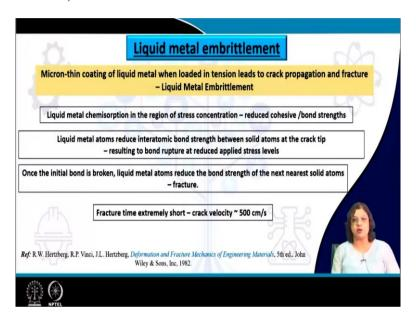
So, moving on to the next topic which is liquid metal embrittlement. What it says is that the micron thin coating of liquid metal when this is loaded in tension that leads to crack propagation and fracture that is what is a liquid metal embrittlement. So, we have one material over which there is a coating which is very, very thin of the order of few microns or even sub microns.
