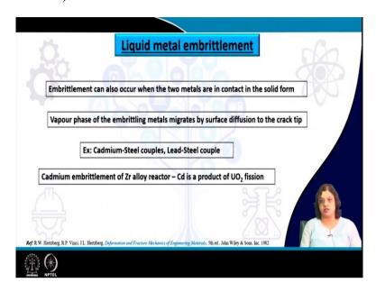
Now, liquid metal embrittlement can also occur when the two metals are in contact in the solid form. The vapor phase of this embrittling metals whichever is in the top which is forming this coating that migrates by surface diffusion to the crack tip or for that matter any other stress concentration side. Now, there are some examples that we should be concerned about. For example, the cadmium-steel couples or the lead-steel couple is a very, very reactive.
