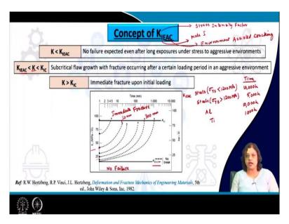
So, there comes the concept of  $K_{1EAC}$  so the 1 here signifies mode 1 let me also write down the K here. So, K is nothing, but the stress intensity factor and EAC of course is environment assisted cracking. So, this signifies the critical value of the stress intensity factor at which material or component or a structure will fracture in presence of certain combination of environment or combination of different metals.
