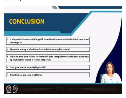
So, here are the conclusion for this lecture. It is important to understand as I mentioned the specific material environment combination that is more prone to undergo stress corrosion
