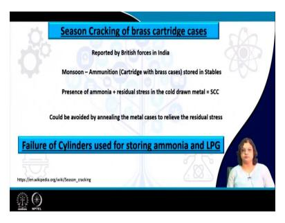
So, this is an incident known as season cracking which has happened in the dependent India which was under the British force at that time and this was reported by the military forces to the British government at that time that there was just cracking of the brass cartridge that is used like the cartridge that is used typically has a cover of brass. So, it just keeps on cracking on its own and that sometimes lead to some explosion also and could be quite catastrophic.
