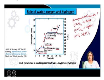
Now, this graph here very interestingly shows how the crack growth will behave or will occur with respect to time in different conditions. So, let us see how it behaves in presence of the humidified argon. So, argon anyway we are well aware that argon is a medium through which if there is an inert medium through which the crack or any kind of reaction is not supposed to happen.
