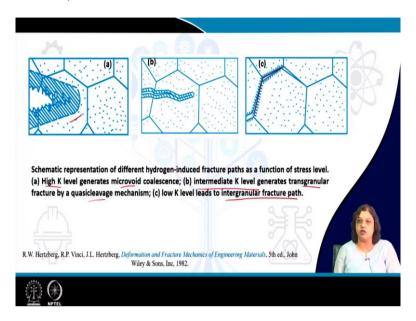
But wherever it is if we are changing the values of the stress intensity factor that can also change the mode of fracture as well. So, presence of the hydrogen while it generates the internal stresses and that will aggravate the situation of the cracking process if we are applying higher values of stress intensity factor that leads to early onset of the micro voids and then this micro voids with coalescence and that will lead to the progress of the crack as has been seen in this figure here.
