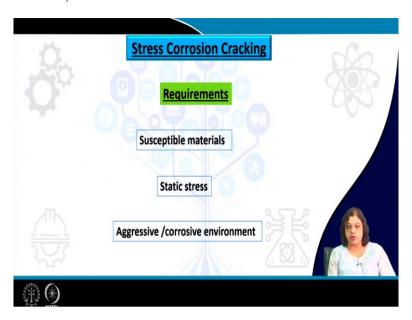
And now let us move on the stress corrosion cracking. Now, stress corrosion cracking is another way by which material or system component can fracture at a lower values of stress intensity factor then what is applied and the particular requirement or particular factors that are required to have this materialize the stress concentration, stress corrosion cracking are the following.
