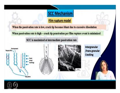
So, typically this is also related to the passivation rate the growth of the crack. When the passivation rate is low crack tip becomes blunt due to excessive dissolution, the corrosion reaction is happening and that leads to dissolute the material and that makes the crack tip blunt. Now, if the crack tip is getting blunt obviously the stress concentration factor reduces there and that means that the amount of plastic zone or the ability to plastic deformation also reduces.
