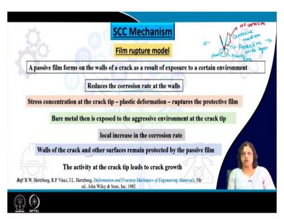
And what typically happens is the passive film forms on the wall of the crack as we have seen if there is a crack here. The passive oxide forms at the crack surfaces when this is so this is the corrosive medium and this is the crack. So, we have a protective or passive oxide layer this could be just the product layer and that prevents the crack or the material from further corrosion to occur that reduces the corrosion rate at the walls that is fair enough.
