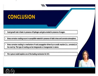
So, coming to the conclusion for this part of the lecture what we have seen is the crack growth rate is faster in presence of hydrogen and it gets completely arrested while there is oxygen. Stress corrosion cracking occurs in a material which is susceptible to undergo corrosion in presence of static stress and the corrosive atmosphere. So, all these three factors the corrosive atmosphere, static stress as well as the material which is susceptible to undergo corrosion reaction.
