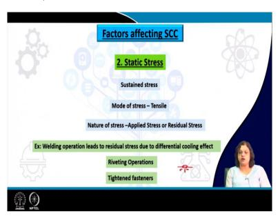
The second factor is the static stress. The stress need not be cyclic it may also happen with cyclic loading or fatigue loading, but even if this is just a static stress which means that there is a continuous application of a particular amount of stress, particular magnitude of stress that is also sufficient for stress corrosion cracking to occur. So, this stress has to be sustained and the mode of the stress that actually will lead to stress corrosion cracking is tensile.
