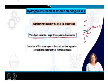
So, there are different ways by which this hydrogen embrittlement occurs. One of this is the hydrogen environment assisted cracking or HEAC. So, this signifies that hydrogen is introduced at the crack tip by the process of corrosion. So, this hydrogen comes as the corrosion product and at the vicinity of the crack tip because of the presence of large stress there is of course some plastic deformation that happens.
