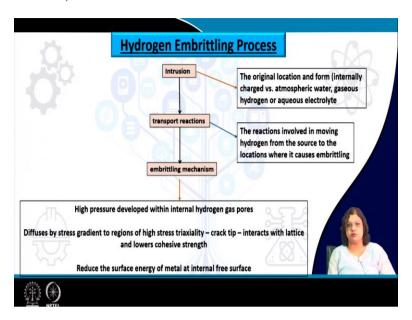
So, based on this let us just summarize this embrittling process. So, first of all hydrogen needs to be included in the system and this is related to the original location and form particularly whether it is internally charged or it has come from the atmospheric water or gaseous hydrogen or aqueous electrolyte this dictates that how the hydrogen will form and how the hydrogen will include in the system.
