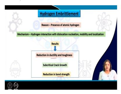
So, let us move on to the first one; hydrogen embrittlement. As I mentioned or as the name suggests that hydrogen embrittlement is particularly related to the presence of atomic hydrogen and hydrogen in the atomic form is what is needed that leads to all the reactions to occur and that leads to the final failure. So, the mechanism more or less depends on the interaction of the hydrogen atom with the dislocations, the nucleation of the dislocation, mobility as well as localization process.
