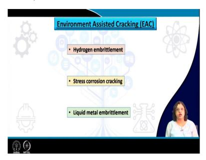
So, what happens in reality is that often we determine the plane strain fracture toughness of a material and then in actual practice it fails at a much lower values of the  $K_{1C}$  or the fracture toughness values are quite less than whatever is expected or whatever is determined from the lab scale testing. Now, this is particularly one of the reasons is the fracture behavior being aggravated by the environmental conditions.
