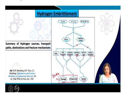
So, this is the hydrogen embrittlement in short. So, it shows the summary of the hydrogen sources so let us see what could be the sources that we have discussed. So, either there are this gaseous hydrogen which is dissociated into the atomic hydrogen or there are this hydrogen ion which again forms this atomic hydrogen because of some reactions or the corrosion reaction.
