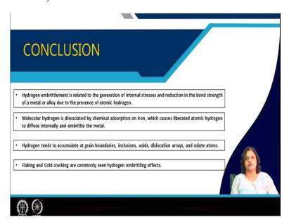
So, let us conclude this lecture here with the following points that hydrogen embrittlement is related to the reduction in bond strength of a metal or alloy due to the presence of atomic hydrogen and this occurs by several steps. First of all, the molecular hydrogen is disassociated by either chemical absorption on iron or there could be some corrosion reaction as well that causes the liberated atomic hydrogen to diffuse internally.
