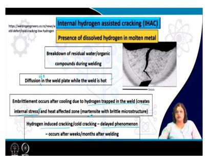
Now, let us see what are the other mechanisms of this internal hydrogen assisted cracking. As I mentioned that IHAC is considering that the hydrogen is already dissolved in the molten metal and this can also happen by the breakdown of the residual water or if there is some organic compounds during the welding that may breakdown and that lead to the presence of the hydrogen.
