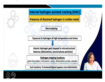
Hydrogen can also come from the electroplating. Now, this is an irony since electroplating is mostly used to have the material higher corrosion resistance, but that itself can insert or include the hydrogen in the system or in some cases if the component if we know that this is in service in the hydrogen atmosphere in presence of high temperature and stress so that also lets the hydrogen to enter into the system that high temperature and stress facilitates the hydrogen to enter into the system.
