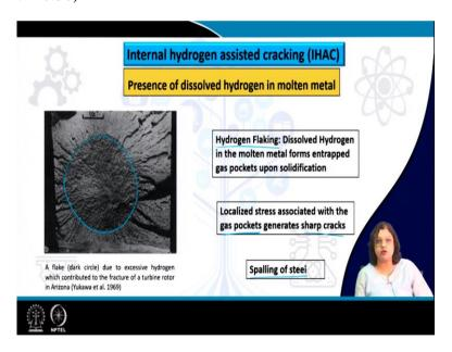
There are another way other than the environmental hydrogen there are the internal hydrogen that also can lead to the embrittling of the component which is known as internal hydrogen assisted cracking. So, this signifies the presence of dissolved hydrogen in the molten metal or hydrogen is already existing in the system and one of the significance or one of the very commonly found defects or hydrogen embrittling defect is hydrogen flaking.
