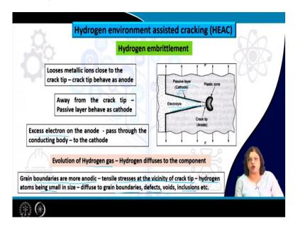
In fact, the metallic ions which are close to the crack tip that is being lost and that serves as the anode. So, the crack tip itself serve as the anode. As you can see here that because of this plastic deformation here this protective layer gets ruptured and that lose some metallic ions making it a anode. On the other hand, the other part the wake of the crack particularly which is covered with this corrosion product layer that serves as the cathode layer.
