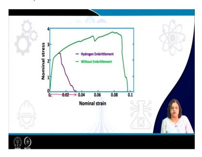
As you can see so if we are considering the stress strain behavior of a material and the green one here signifies the experimental stress strain behavior of a material which shows quite a bit of ductility. On the other hand, because of the presence of hydrogen in the atmosphere and because of the hydrogen embrittlement to be active for the same material we see that the ductility has been reduced notably.
