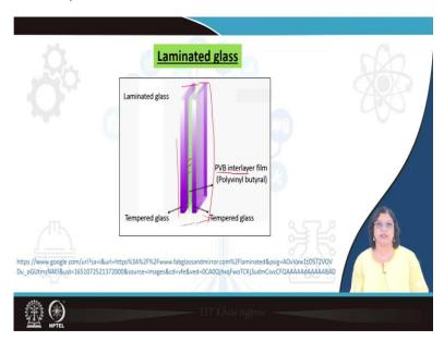
So, this is how it is done this are the tempered glass can be used one which is already tempered by thermal or chemical way and then in between if we are using this polymer sheets here, so, in this case, this is a PVB that is shown here and if you make a sandwich structure and this entire one is a laminated glass, which is used for making some kind of component. So, if we are using that the toughness will be increased to a very high extent.
