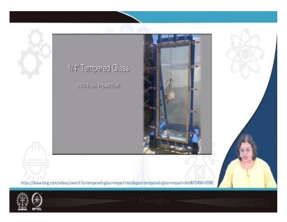
So, the concept that will be covered in this lecture is continuing with the toughening mechanism of glasses and then we will also look into the different factors that controls the toughness of even polymers. So, here is a small video which shows that how a glass which is toughened by tempering does not even break even if we are applying impact loading on this. So, this one is interesting video which kind of represents what we have seen in the last lecture.
