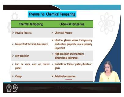
So, this certainly has a significant influence. Let us just look onto the differences between the thermal and the chemical tempering. First of all, thermal tempering is a physical process we are simply heating it above the glass transition temperature and cooling it so we are not altering or modifying the composition in any way.
