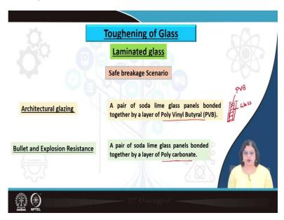
So, a laminated glass is often used for architectural glazing, in which case a pair of soda lime glass panels, so we have two pieces or two sheets of soda lime glass and that is bonded together by a layer of PVB, polyvinyl butyral. So, it is a kind of sandwich structure in which there are two layers of glass. So, there is two other glass layers and then there is this BVB that is a polymer that is used for sandwiching this glass plates or sheets.
