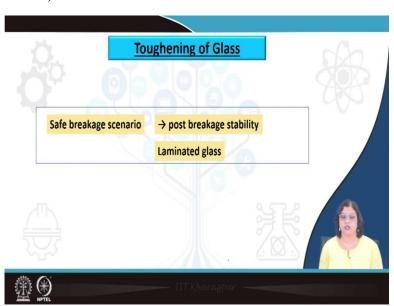
Now, so, that was no break scenario. And the next one that we are going to discuss about now is the safe breakage scenario. So, in this case, although if the glass component breaks, there should be some mechanism of load sharing such that the entire component should not fail catastrophically and this can be obtained by different way and so that we can achieve a post breakage stability although the glass breaks, but there could be some stability of the structure
