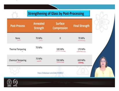
This is an example of how different kinds of toughness can be achieved or strengthening can be achieved just by tampering. For example, if no tempering operations are being done, we see that if the annealed strength of the glass component is 70 MPa, the final strength is also the same because there is no additional residual stresses in the glass.
