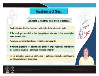
The reason for this is the fact that this laminate actually should act along the crack or arrest orientation. So, it should be positioned in such a way that the crack growth direction should be hindered and it will act as a crack arrestor. We have also discussed about the crack arrest morphology in the previous lectures and you can very well imagine that all this the sandwich
