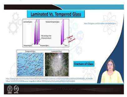
Now, let us look into the differences between the laminated versus tempered glass. So, this one is the standard tempered glass here as we have seen that this tempering can be achieved by either thermal or chemical way. On the other hand, laminated glass may use this tempered
