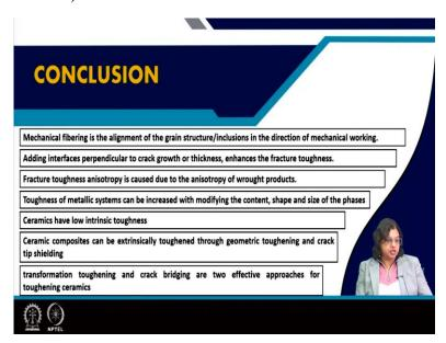
So, let us conclude this lecture with the following points here. What we have seen is that mechanical fibering is means that it aligns the grain structure or the micro structures in general including even the inclusions along the direction of the mechanical working and adding interfaces perpendicular to the crack growth or to the thickness direction enhances the fracture toughness.
