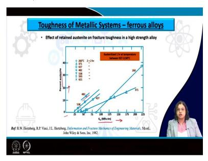
Now, for the case of metallic system, if we try to enhance the fracture toughness of metallic system, let us first go with the ferrous alloys, because this is the one iron base alloys are the one which are most commonly used to structure materials for the metallic segments. And for that one of the ways by which the toughness can be enhanced is by having higher amount of austenite retained austenite phase.
