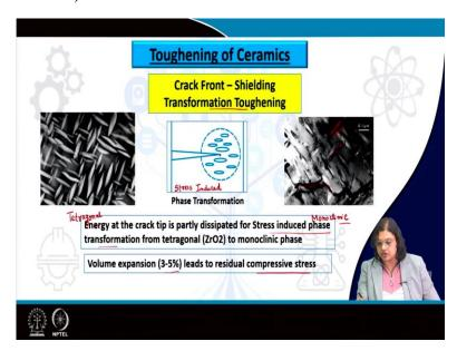
So, we will look into two of these different ways by which the fracture toughness can be increased one is the crack front shielding that we have seen this one is very important particularly for ceramics, but also seen for metallic system which is the transformation toughening. So, what happens here is that at the tip of the crack because of the presence of high amount of energy there that can lead to some stress induced phase transformation.
