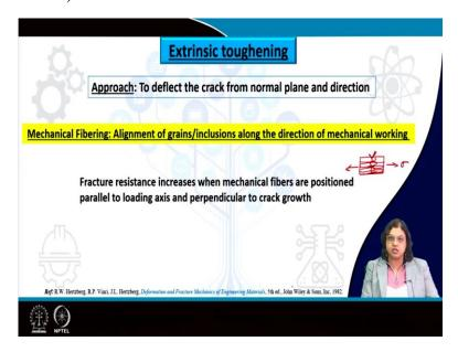
So, coming to the point of view from the extrinsic toughening, we know that this is the way by which we deflect the crack from its original plane and direction of motion to another one we kind of diverted and part of the energy is consumed in all this diversion, which enhances the total energy consumption and that means, the fracture toughness of the material increases.
