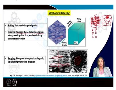
So, let us see how this mechanical fibering looks like? the typical operations that we do the mechanical working that we do are rolling and due to the rolling, what we achieve is elongated grains along the direction of the rolling. On the other hand, one that we otherwise use other than rolling is drawing we often need to draw for example, for wires or rods, we often need to draw it along some particular direction.
