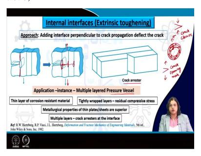
And the other very interesting way by which toughness can be enhanced extrinsically is by adding some surfaces, free surfaces which means that if we are making some layers in the component, then we can still achieve higher toughness providing that those interfaces or those layers are perpendicular to the crack propagation direction and that essentially will lead to deflection of the crack.
