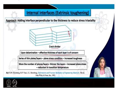
Another way by which these internal layers can actually lead to an enhancement in toughness is by adding this interface perpendicular to the thickness direction and this is known as crack divider where you see that instead of having the layers along this direction, we are having the layers which are perpendicular to the thickness direction and that is also beneficial in the sense that in this case, the crack growth direction is not being hindered by the interfaces.
