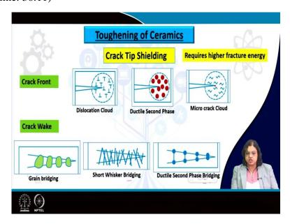
Now, other mechanism of toughening in ceramics include crack tip shielding. So, this means that we if there is a crack already existing and if the tip is being shield by some other
