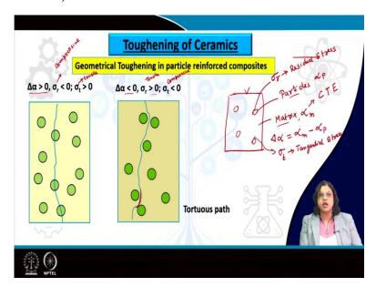
Now, in case of the particle reinforced composite, let me draw it here. So, if we have such kind of behavior where we have a matrix phase as well as these are the particles or precipitates. So, what is of interest here is the coefficient of thermal expansion for these particles as well as the matrix. So, if we denote this with the symbol  $\alpha$ , so, this signifies the coefficient of thermal expansion.
