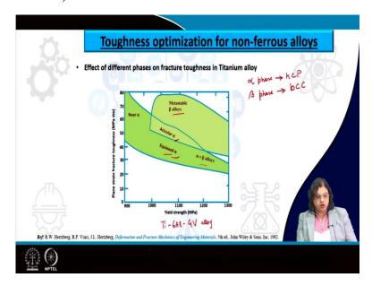
Now, for the case of non ferrous alloys, here is one example of titanium alloy, now titanium alloy so, this one is actually a Ti-6Al-4V alloy that has been shown here and there are different phases in this titanium system also for example, the  $\alpha$  phase which has a hexagonal close packing structure as well as the  $\beta$  phase which is having a body centered cubic structure and it is seen that the  $\beta$  phase particularly the metastable  $\beta$  phase has the highest toughness.
