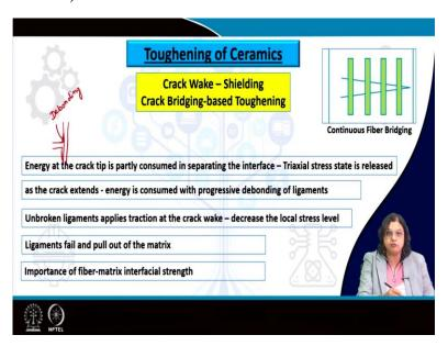
The other way by which ceramics can be toughened is through the crack wake shielding and that is by the crack bridging. So, what happens here is if we have this is particularly for the fiber reinforced composite, if we have a fiber like this and then there is a crack coming. So, it is possible that it is getting D bonded here at the interfaces and because of this D bonding once again the toughening the fracture toughness of the material is going to increase.
