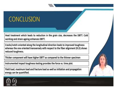
So, as a conclusion to this lecture, we have seen that any kind of heat treatment which leads to reduction in the grain size or grain refinement actually leads have a positive effect and it leads to reduction in the ductile to brittle transition temperature.
