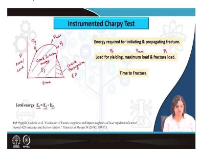
First of all, what we can determine if we are getting the force versus time curve is something like this. So, we can see that if we are having this load or force versus time what we can see is a behavior something like this and can fracture. So, basically, we can find out the load that is required for yielding, let us name this as  $P_y$ . So, this is the load for yielding at which the yielding behavior of the specimen has started.
