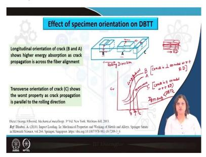
Now, another important way by which DBTT can be controlled or which typically shows some effect on the anisotropy of the behavior is the specimen orientation. Now, this is an example shown here, this is a rectangular billet or some structure which has been rolled along this direction, so, this is the rolling direction. And if we have some rolled structure, we also know
