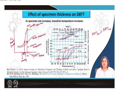
Now, apart from the orientation, thickness also has a major influence on the ductile to brittle transmission temperature and what we can see here from this slide, we can see that there are some experimental results shown for the different thickness of material starting from thickness of 1.25 up to 15 millimeter and very clearly if you look into this the curves below are in
