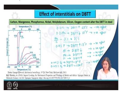
But, what we have more control on is the effect of the interstitial atoms that are being added for purpose. Now, there are of course, different need for which we add the interstitial atoms. Let us focus on some of the commonly used interstitial atoms which are used particularly for steels different grades of steels and which have some role on the ductile to brittle transition.
