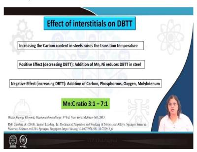
So, in a gist what we are seeing here is that increasing the carbon content in steel raises the transition temperature and there are of course elements like manganese and nickel which has positive effects. Whereas, there are elements like apart from carbon, there are phosphorus, oxygen, molybdenum, which has a negative effect on the ductile to brittle transition which means that it increases or enhances the DBTT.
