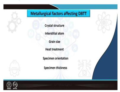
Our next target as metallurgist or as an engineer would be to control that, we want to know the mechanism behind any kind of mode of fracture with the primary aim to control that, to manipulate that based on our service requirements. So, that we can change this DBTT as per the requirement and then we can achieve the expected performance of a material. So, of course, there are different ways by which we can control that or we can modify that and the first one is the crystal structure.
