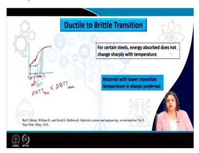
Apart from that, let me also indicate that as I mentioned this ductile to brittle transition behavior changes from materials to materials. So, for certain steel this energy absorbed does not change very sharply as well as for some cases there is a very drastic change in the failure mode. For example, if we are plotting this once again as the C<sub>V</sub> versus T we can see that for some kind of steel it is following a very drastic change.
