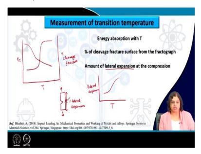
So for that case the transition temperature is determined based on the following ways so first of all let me once again draw this, so this is the energy versus temperature and as we mentioned that this shows a typical S kind of curve that there is an upper shelf and there is a lower shelf, now this is the energy variation if we are not talking about the percent cleavage fracture.
