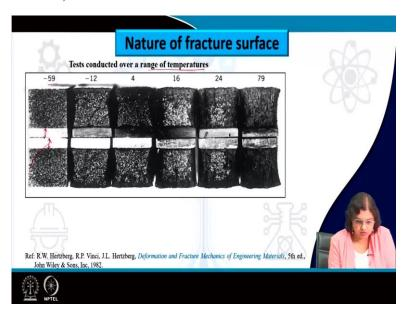
But we always try to find out the quantitative value for that so that we can specify the amount of ductility or the amount of brittle mode there. So for that we actually need to perform a series of test and to figure out this kind of the S shaped curve that we have seen so far. So, here are some examples of the fracture surfaces for both the pieces after fracture and this has
