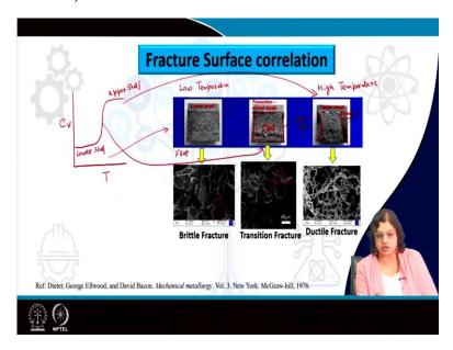
So, if now, we try to correlate this with the energy diagram, once again let me draw this in parallel. So, this is the energy and this is the temperature and we are very well seeing the upper shelf and the lower shelf, this is for a case when it shows a very distinct ductile to brittle transition mechanism.
