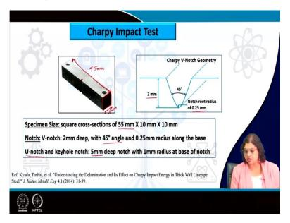
So, coming to the Charpy impact test, this is the kind of specimen that is particularly used here and the specimen size and all the different geometrical parameters has been standardized already and this is the kind of specimen where we use the total length. So, let's say this thing
