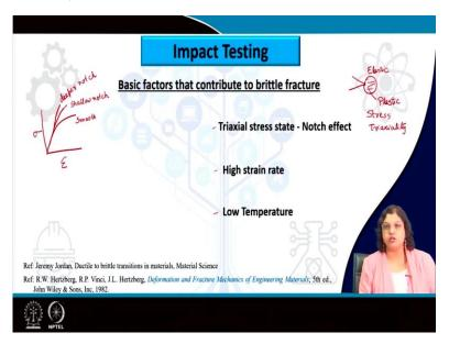
So, if that is the case, we need to figure that out through some testing and there comes the major factors that are of concern for the case of impact testing. So, impact testing was first thought about by Charpy, long back in around 1912, and all when all those failure things are happening, people came to know about the importance of the different factors that could have led to the failure and designed and experimental way to find out the toughness of a material.
