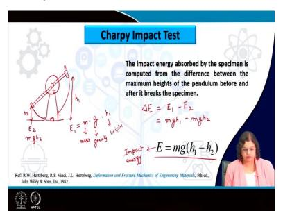
So, let us see how the Charpy impact test is typically done. So, what we have here is a dial and with this is a pendulum or a hammer. So, this is the base of the instrument in which the specimen is being kept. Now, this hammer hits the specimen like this to the specimen and then it stops after certain distance, the specimen flies up it breaks or it gets deformed.
