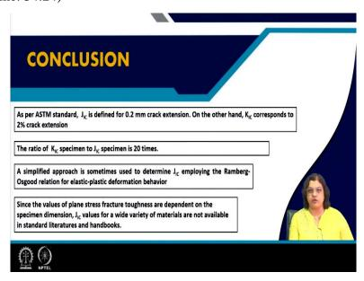
Let us conclude this lecture with the following points, which are the take away thoughts from this lecture which says that the  $J_{IC}$  is defined for 0.2 millimetre crack extension that we have seen, and the ratio of the  $K_{IC}$  specimen to  $J_{IC}$  specimen is 20, which makes a  $J_{IC}$  specimen quite large.
