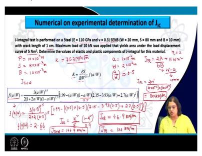
So, let us just solve simple numerical to make this idea a little bit more clear. So, here is an example for a steel component, an SENB a single edge notched component, which has the elastic modulus and elastic modulus of 110 GPa and the Poisson's ratio is 0.3. And the other parameters for the SENB specimen are as follows. The width is given as 20 millimetre, span length, which is the distance between the loading point as 80 millimetre.
