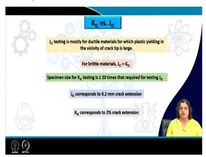
Now, moving on to the next part, let us see that how  $K_{IC}$  is different from that of  $J_{IC}$ . First of all, we have seen that,  $J_{IC}$  testing is mostly used when we are talking about ductile material and when there is a significant amount of plasticity and plastic yielding in at the vicinity or in the at the tip of the crack, which is very, very large, and we cannot ignore it.
