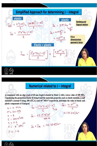
So, here is a numerical related to that, which says that there is a component with an edge crack of 40 millimetre length. So, that makes the, a value, as let us say, 0.04 meter. And this is loaded in mode I with the stress value of 200 MPa. So,  $\sigma$  equals to 200 MPa, and the geometric factor H is considered as 8. And the material property such as the elastic modules in. So, elastic modules is 200 GPa.
