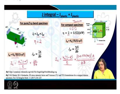
So, again as I mentioned that the  $\eta$  factor is dependent on the specimen dimensions and the specimen configuration. So, let us see this for the two most important configuration or most
