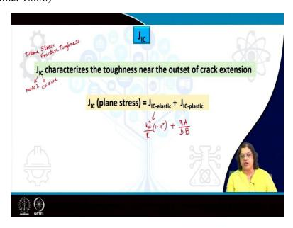
And from there we can calculate not only J integral, but more specifically  $J_{IC}$ . So,  $J_{IC}$  characterizes the toughness and crack tip at near the outset of crack extension. So, this once
