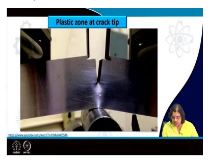
So, this is being maintained. And you can see here that there is the plastic zone which is forming at this point here. So, that signifies the plastic deformation and if you look that carefully, you can see that there is a crack tip blunting as well. So, initially the crack was even sharper and just in this clip itself, we can see that the crack tip is getting more and more blunt. So, basically the effective crack length is increasing.
