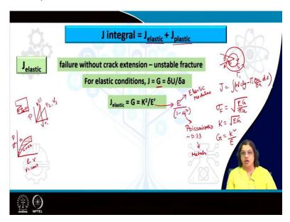
So, in the last lecture, we have seen that J integral is basically obtained for any contour and let us say we have a crack tip and we are talking about a contour in the immediate vicinity of this crack tip such that this is  $\Gamma_1$  and starting from the point A and moving to B and then C with another contour, the direction of which, the direction of motion being opposite to that of the  $\Gamma_1$ . And finally, the surface segment D A is closing it.
