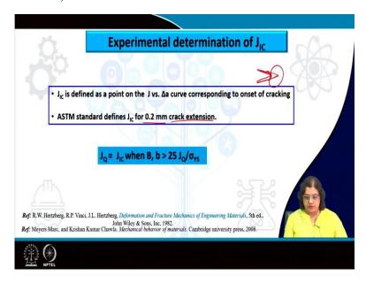
Now, this is not arbitrary, it is not or whim that we can see that we have to maintain this ratio, there might be some particular reason for this. And the reason is that, we have to appreciate this that in case of plane stress fracture toughness, whenever there is a crack and a plastic
