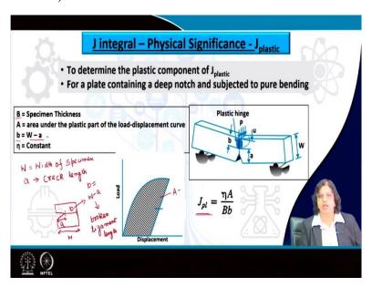
On the other hand, when we are talking about the plastic part, we still need to consider the area under the curve and for that case, let's say in case when a specimen is being subjected to pure bending something like this, we can obtain the plastic part also and the area under the plastic curve is determined as A which is the area under the plastic part of the load displacement curve.
