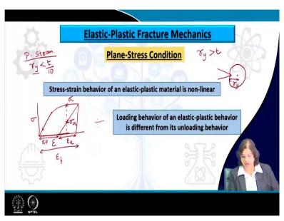
So, let us begin with the first topic itself, which says the elastic plastic fracture mechanics and this is particularly valid for the plane stress condition. So, so, far we have seen that how a material behave or fail in a brittle fashion, when it undergoes failure or fracture in the plane strain condition. And we have seen that Griffith criterion is being followed for most of the cases, so, that we can estimate the fracture toughness or fracture strength according to that relation.
