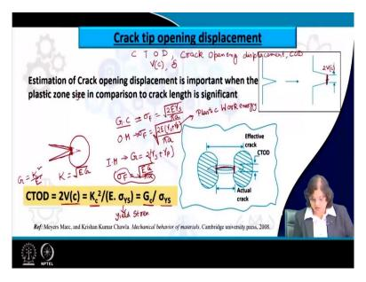
So, one of the typical way by which this can be analyzed to some extent is the crack tip opening displacement also known as the CTOD. Sometimes, also this is considered as or this is termed as crack opening displacement or COD. So, what does this mean crack tip opening displacement, so, essentially it means that something is happening to the tip, the tip gets opened up.
