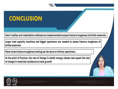
So, with this let us conclude this lecture. So, what we have understood here is that, the short rod or bar and indentation methods are some of the other ways by which we can estimate the fracture toughness particularly for brittle materials, these are advantages considering that we do not need a complicated specimen dimension or higher load capacity machine.
