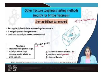
So, with this let us move on to some other methods by which fracture toughness is measured particularly for brittle materials. Now, the problem that we cannot use the method that we have discussed in the last lecture is that in case of brittle material, it is very difficult to machine a notch or certain configuration. So, that is why we go for a little bit simpler method where the specimen preparation is not that difficult to go ahead with the fracture toughness testing.
