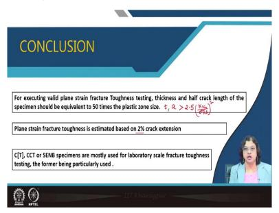
So, that leads us to end of this lecture, which says that for executing a valid plane strain fracture toughness testing thickness and half crack length of the specimen should be equivalent to 50 times the plastic zone size and this is what we are getting that this t,a  $> 2.5 \left(\frac{k_{IC}}{\sigma_{YS}}\right)^2$ . So, this 50 times of the plastic zone size actually is coming as 2.65 and we are simply rounding it up to the value of 2.5.
