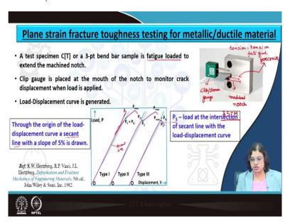
Now, let's see the details of how the fracture toughness testing is being performed in lab under plane strain condition. So, initially CT specimen or a compact tension specimen or a 3-point bend specimen or sometimes even a center cracked tension specimen are used for fracture toughness testing and all these specimens are having a machined notch.
