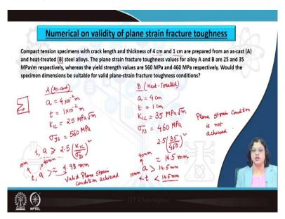
So, let's see based on a numerical that how we can practically do that in case of material, which might have different values of fracture toughness or yield strength of the material. So, here is the compact tension specimens with crack length and thickness of 4 centimeter and 1 centimeter
