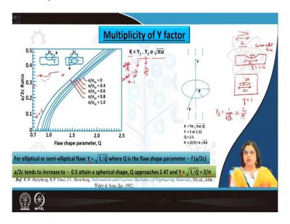
Now, along with that we also need to consider the shape of the flaw. So, so far we have seen that there are notches which are either machined or change in the parameters of the the geometry which leads to a sharp crack. And for that we considered particularly the crack length or half crack length being a.
