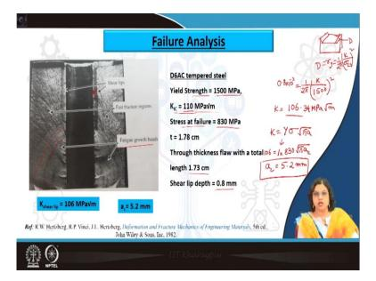
So, before we move on, as we have seen in the last lecture that whenever there is a fracture from the fracture surface itself from the fractograph, it is possible to determine the fracture toughness at the point of fracture and this is done typically considering the shear lip width. So, if this is the shear lip width, which typically occurs because of the plane stress condition, we can determine the shear lip width.
