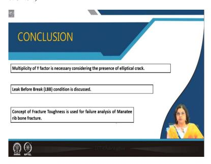
So, let us come to the conclusion for this lecture. What we discussed here is the effect of this multiplicity Y of Y factor due to the presence of elliptical or semi elliptical crack. And we have also considered or discussed about the leak before break condition and how that can be generated, how to take care of this factor while designing a component for such critical application. And the concept of fracture toughness is used for the failure analysis of manatee rib bone fracture.
