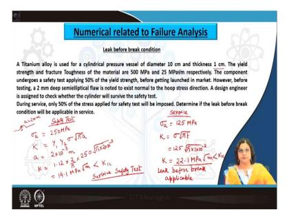
So, let us do a numerical to make this clear. What it says is a titanium alloy which is used for a cylindrical pressure vessel, which is having a diameter of 10 centimeter and thickness of 1 centimeter. The yield strength and fracture toughness of this material are 500 MPa and 25  $MPa\sqrt{m}$ , respectively.
