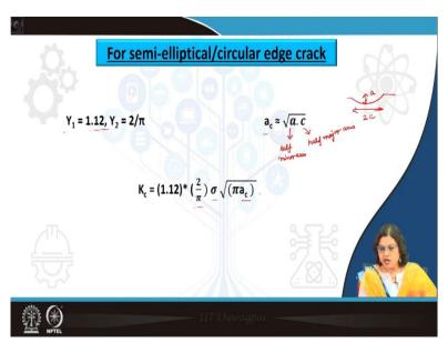
So, this is what is shown here. So,  $Y_1$  as 1.12 for the case of edge crack and  $Y_2$  is  $\frac{2}{\pi}$ . So, this is typically for semi elliptical or semicircular edge crack. Now, if we have a elliptical one and in which case the c and the a are distinctly different numbers and it is not semi circular but semi elliptical, in that case, we often needs to find out the  $a_c$  value.
