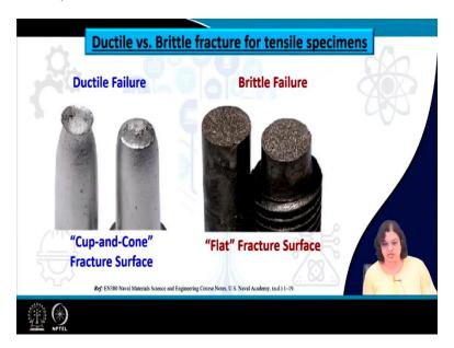
If we look into the fracture surface on the specimen, this is how it looks. So, this is a tensile specimen means the specimen has been tensile tested and what we can see is a typical cup and cone kind of fracture you can see that this takes the shape of a cup and this takes the shape of a cone. So, this is how the fracture surface of a typical tensile specimen looks like.
