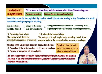
So, recrystallization; as I said consists of nucleation. So, giving emphasis on nucleation during recrystallization phenomena; so, nucleation in recrystallization. So, the critical factor to determine both size and orientation of the resultant grain. So, nucleation is the critical factor that determines both the size and the orientation or the texture of the resultant grain.
