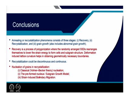
So, what we understood from this lecture class is that one, annealing or recrystallization phenomena consist of three stages right; recovery, recrystallization and grain growth. It should also include secondary recrystallization, which is abnormal grain growth right. Recovery is a process of polygonization, where randomly arranged statistically stored dislocations rearranges themselves to lower the strain energy to form cell and subgrain structure.
