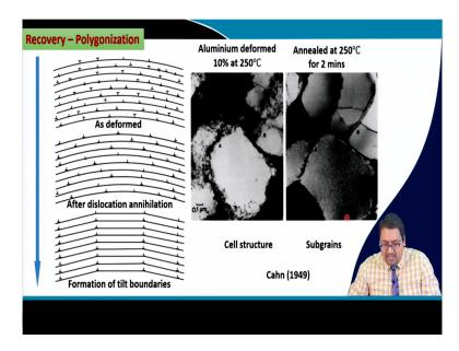
So, recovery as explained earlier is a process of polygonization. So, polygonization is a process, where you see any deformed material contains statistically stored dislocations. So, you can see there is there are lots of dislocation present throughout the microstructure and now, because of the plastic deformation induction in the material and the presence of multiple
