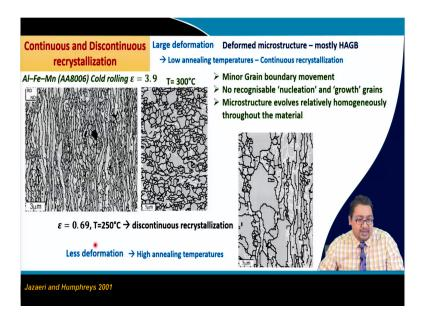
Now, let us say how in static recrystallization phenomena a continuous and a discontinuous recrystallization looks like. Let us take an example of aluminum Fe-Mn known as AA8006 alloy, cold rolled to a strain of 3.9. So, a large deformation is given. So, deformed microstructure, we can see; elongated microstructure could be observed. So, the vertical is the RD and the horizontal direction is the ND. We are looking in the TD direction as usual transverse direction.
