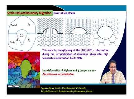
So, you see there is another model of recrystallization and this is a strain induced boundary migration model. And such kind of situation is mostly observed in low initial strain conditions. So, low deformation condition. Such a model states that as the deformation as the deformation is not heterogeneous as I explained in few slides before.
