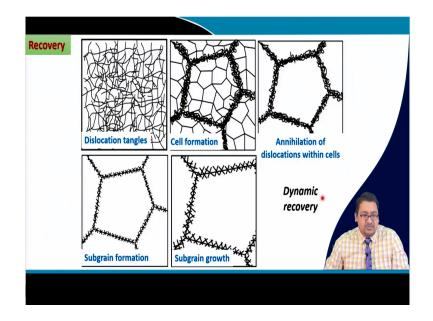
So, recovery process; so, recovery process consists of basically the presence of dislocations or dislocation tangles being randomly present throughout the cold deformed cold plastically deformed microstructure and the formation of cell structure with diffused dislocation wall ok having a high density of statistically stored dislocation at the boundaries, and the low density of statistically stored dislocation inside the cell.
