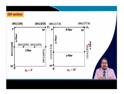
So, we have shown the ODF section of phi 2 equal to 0 and phi 2 equal to 45 degree section with phi 1 0 to 90 degree phi 0 to 90 degree in both the cases. And to let you know that because of the crystal symmetry the phi and the phi 2 is reduced from 0 to 360 degrees to 0 to 90 degree in case of body centered cubic material whereas, because of the rolling symmetry the phi 1 is reduced from 0 to 360 to 0 to 90 degree in this case.
