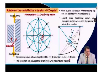
Now, this slide shows the utilization of the 100 stereographic projection in observing the rotation of the crystal lattice when tension or a tensile test is conducted in a face centered cubic crystal. One can show the same thing for tension in a BCC also compression in FCC
