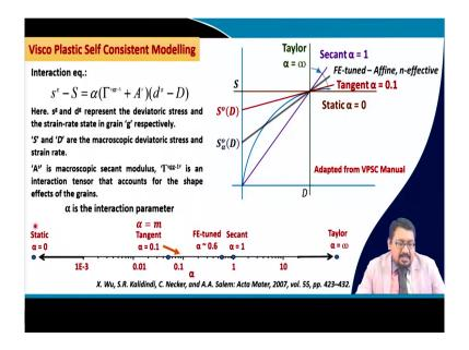
So, if we look into one of this model, the visco plastic self-consistent model, which are being used in a large scale by various researchers in this area to understand the texture evolution and the strain hardening behavior it the model consists of mainly two equations; one is the interaction equation.
