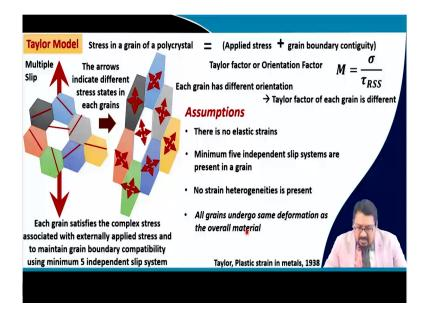
Now, comprising of the Sachs model, where we considered a polycrystal material with grains having different orientation. In this case also, we will take the same condition where there are multiple grains in a polycrystalline material and each grain comprising of a different orientation.
