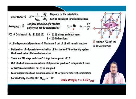
So, Taylor factor as I said M is given by sigma by tau R S or d gamma by d epsilon x depends upon the orientation of each grain right and can be calculated for all the orientations.
