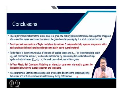
So, from this lecture class, we can conclude that the Taylor model states that the stress state in a grain of a polycrystalline material is a consequence of applied stress and the stress associated to maintain the grain boundary contiguity. And it is a full constraint model.
