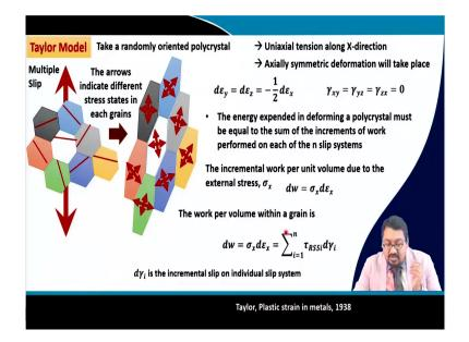
So, the if we take a randomly oriented polycrystal and give a tensile deformation to it as we are given, then let us say that uniaxial tensile is giving in the X-direction. And so, as the texture is random as the polycrystalline material is randomly oriented polycrystal.
