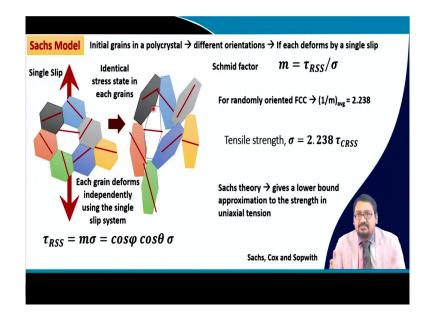
So, if we look into the Sachs model. The Sachs model considered that initial you know grains of the polycrystalline material. Say for example, these grains are having different textures. So, they all have different orientation. And each deformed by a single slip as single crystals present in this polycrystal.
