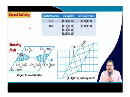
So, if you look into the most of the crystal structure in metallic materials are either face centered cubic material or body centered cubic materials. Few, like magnesium, titanium, zinc, zirconium, also have an hexagonal close packed structure.
