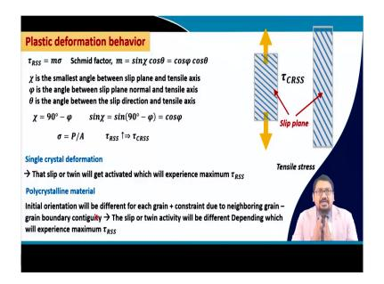
So, if we look into the plastic deformation behavior for a single crystal say for example. And if we say that yes this is the sample that we had, and this is a single crystal, and we tried to pull it by a tensile loading, and say that these are the certain slip plane which starts to get activated, there could be various slip planes.
