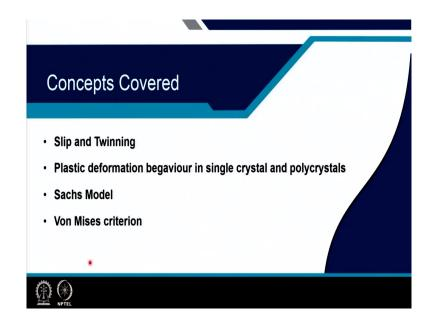
So, the concepts that will be covered in this lecture are slip and twinning mechanism in formation. Plastic deformation behavior in single crystals and in polycrystals. And we will cover Sachs model which is basically comprising of utilizing Schmid factor for a certain Schmid slip system to observe the you know plastic deformation. And then, finally, the Von Mises criterion.
