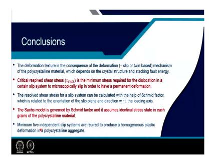
So, we can conclude here that the deformation texture is a consequence of the deformation mechanism which could be slip type, twin type, combination of this and it depends upon the stacking fault energy of the material and it also depends upon the crystal structure. So, this decides that how, what the texture or the deformation texture will evolve.
