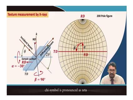
And once we rotate it once we rotate it and increase the beta from 0 to 90 degree the sample is rotated like this . And when the sample is rotated now the TD is here and the alpha is basically sorry the RD goes here right. So, the ND remains the same the position of the ND
