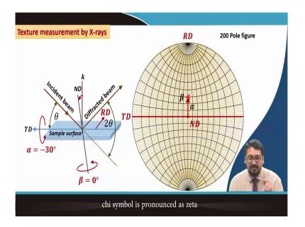
So, when we reach alpha equal to 30 degree we are here and we are observing the intensity at k that is bisector between incident and the diffracted beam which is this position this position right, alpha equal to 30 beta is equal to 0 right.
