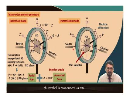
So, while we are talking about the texture goniometer geometry we are showing that we have shown this in terms of the reflection geometry right. In case of neutron diffraction or synchrotron diffraction transmission mode can be also utilized and you can see that there is a subtle difference between the samples which are kept in the Eulerian cradle in case of reflection geometry and in case of transmission geometry.
