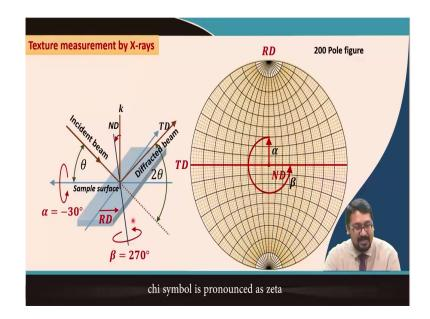
And now, that TD is going backward, where RD is on this side and then we can see that we are tracing the whole sample and we have gone up to 270 degrees.
