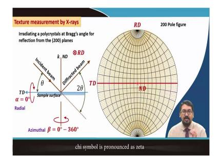
So, let us see how this X-ray texture is being measured. So, we as I said we are trying to measure 200 plane. So, we have kept the theta of that incident angle fixed to 64 4.5 degree based upon the previous diffraction the diffraction experiment in the previous slide right.
