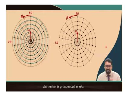
So, here we are showing two methods. This, the left one is the one which was initially done. So, stepper motor was used to vary both alpha and beta slowly and slowly at means different resolution. So, this we have shown very roughly. And so, if we vary it like that a spiral is obtained and there are various points which are shown here.
