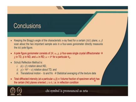
So, we can conclude from today's lecture that if we keep we have to keep the Bragg's angle constant for a particular characteristic X-ray for a certain hkl plane. And then the alpha and beta scan has to be done about the two sample important sample axis that is that is TD and ND in a four-axes goniometer and this directly measures the pole figure that particular hkl pole figure. And this is done for several hkl poles that shows a positive Bragg's diffraction right.
