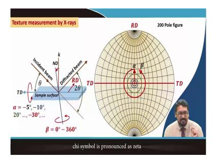
Now, let us say that we rotate the sample by alpha equal to minus 5 degree and why I have said minus 5 degree? Because, we are rotating by clockwise direction that is by the left hand thumb rule. So, what we are getting? We are obtaining a rotation along TD that is alpha equal to minus 5 degree and then while we have rotated by minus 5 degree the ND also will shift from k right.
