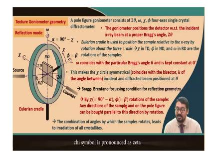
So, that this kind of alpha beta rotation is done using a texture goniometer with a certain geometry. This goniometer, see most of the case is being used in a reflection mode because the X-rays that are produced generally in laboratories are not so intense or does not have the lambda smaller or it is not short wavelength and they are not hard enough to penetrate even the thinnest specimen in order to obtain diffraction pattern from the in a transmission mode.
