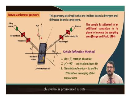
So, that the texture goniometry geometry consists of a X-ray source, a source which has a divergent beam and a convergent diffracted beam. And you in order to make this divergent beam and the convergent beam smaller various kinds of slits are used. horizontal divergence horizontal slit and vertical slits and then receiving slits and anti scattering slits are used in front of the detector.
