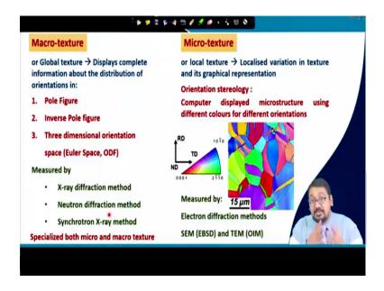
What is macrotexture? Macrotexture is usually called bulk texture or global texture and it displays a complete information about the distribution of orientation. It displays the complete distribution of a orientation in space for a particular poly crystalline material which has been processed by some method right say solidification or deformation or any other method.
