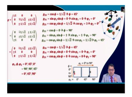
let us take out this g matrix 1, 0, 0, 0, 1 by root 2, 1 by root 2 my sorry, 0, minus 1 by root 2, plus 1 by root 2, 0, 1 by root 2, 1 by root 2. this is RD, TD and ND and we have already have solved that how by rotation of phi 1, phi, phi 2 along ND, RD and ND again to obtain the positions of the Goss components cube components rotated cube components.
