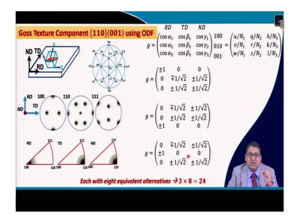
that if we go to the example as I said when we started this lecture that we will show the example of the Goss texture component and which is 110, 001 using the ODF. And, before starting it you should know that Goss texture is a very important texture for electrical steel and it are and this texture is used for transformer.
