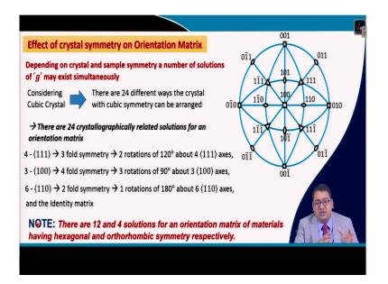
So, that I have said that depending upon the crystal and the sample symmetry, a number of solutions of the g matrix can exist simultaneously right. So, let us consider the cubic crystal.
