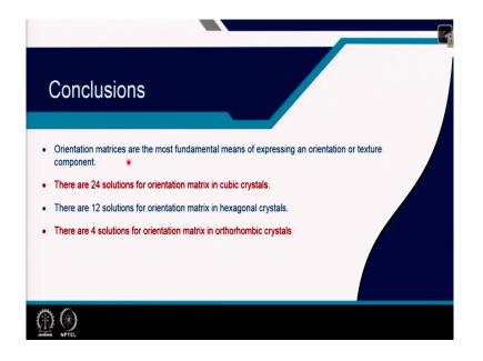
The conclusions are that orientation matrices are the most fundamental means of expressing the orientation or the texture components right. These orientation matrices could be related to the Miller indices via the pole figure or the inverse pole figures right. It could be related to the Euler angles via the Euler space and the Orientation Distribution Functions O D F's. It could be related to the angle axis pair through Rodrigues vectors or Rodrigues space right.
