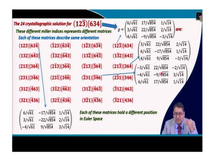
So, that let us go to this cubic crystal and see that for the 1 2 3 bar 6 3 4 kind of texture, how 24 different crystallographic solutions can exist right. So, let us go. So, that if we look into the family of planes for the 1 2 3 right, there could be 1 2 3 bar type plane right, which is this one. And there could be 1 2 bar 3 and there could be 1 bar 2 3, there could be 1 2 3.
