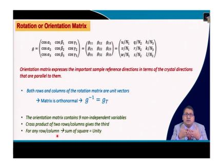
And the orientation matrix, the cos alpha 1 cos beta 1 cos gamma 1. And all the other 9 variables are shown with respect to g 1 1 g 1 2 g 1 3 g 2 1 g 2 2 g 2 3 g 3 1 g 3 2 g 3 3 like this in the matrix. And what are these? And as we have seen that it is the relationship between R D right T D and N D with 1 0 0 0 1 0 0 0 1. Then, we have found out that of course, then this g 1 1 is g 1 1 g 2 1 and g 3 1 is related to R D.
