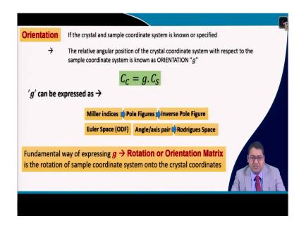
In the previous lectures, we have understood what is an orientation matrix, which is also known as rotation matrix right. So, a orientation matrix is related to orientation right. So, what is an orientation? Orientation is the relationship between the sample and the crystal coordinate system.
