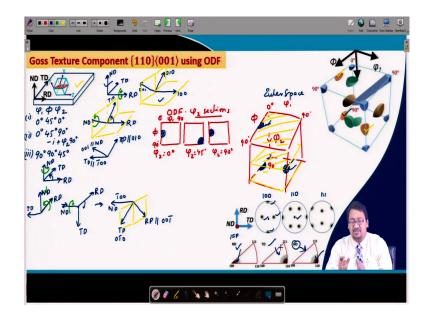
Therefore, ND remains the same, the RD goes to TD and the TD goes to opposite of RD right. Therefore, under this situation the ND remains parallel to 001, the TD that was sorry I have written it wrongly that earlier it was TD and now, it became RD remains parallel to 010 and the TD becomes parallel to 1 bar 00. So, we have traced the specimen axis from the Goss
