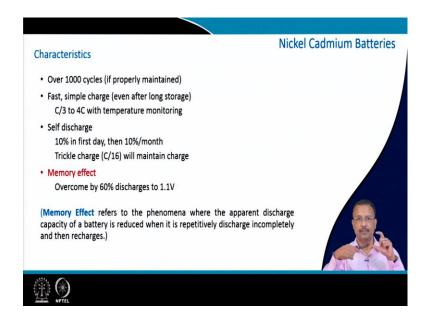
So, if you go through this characteristics a reasonable well cyclability if maintained properly. If you do not have use the battery, you can do a fast charge even 4 C you can charge it. You know that 1 C means 1 hour, 4 C is 15 minutes you can charge the battery. Self-discharge is there. 10 percent per month is a good figure and it has a memory effect that is the problem.
