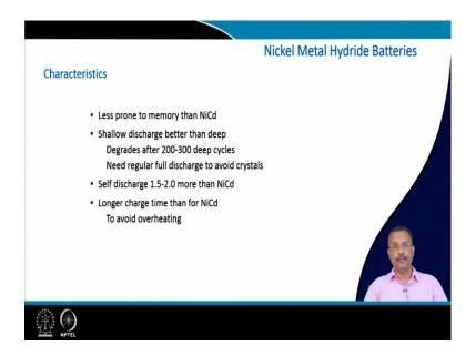
So, they it does not have a memory effect as compared to nickel cadmium. Nickel metal hydride, they do not have the memory effect and one can go to deep discharge and 200 to 300 cycles. It can withstand and self discharge if you keep it in charge condition, then the self discharge is more as compared to nickel cadmium battery and it cannot be charged that fast.
