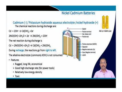
So, nickel cadmium battery, the chemistry is again straight forward what you are using cadmium as your negative electrode and potassium hydroxide aqueous electrolyte that is used and nickel hydroxide that is used as the positive material. So, this is the reaction that takes place in the anode and the nickel oxy hydroxide that reaction is taking place in the cathode. So, the net reaction is and the just the reverse reaction goes from right to left during recharge.
