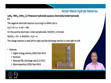
Nickel metal hydride battery, they use of course nickel in the form of various types of alloys and potassium hydroxide aqueous electrolyte is used because it is 1 volt 1.2 volt is the range of voltage that you are getting. So, aqueous electrolyte can safely be used and nickel hydroxide is used as positive material. So, this is the typical reaction that takes place in this positive and negative electrode.
