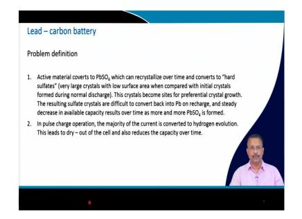
So, if I define the problem of the lead acid battery that is first one is the active material converts to lead sulfate which can recrystallize over time of operation and then basically transfer into a hard sulfate. So, hard sulfate means very large crystals of lead sulfate which are having low surface area as compared to the initial nucleated lead sulfate
