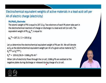
So, now let us see that how this to calculate this active material and it is quite straight forward first you will have to know the atomic weight of lead if you consider lead as a negative electrode material. So, that is about 207.21 gram. So, two electron of each lead atom is taking part in the electrochemical reaction in this system.
