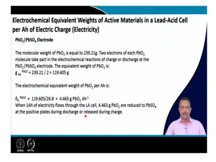
Similarly, you can calculate for lead oxide its molecular weight is 239.21, again two electrons are involved. So, you can calculate the equivalent weight 239.21 by 2. So, that is coming around 119.605 grams. So, electrochemical equivalent weight of lead oxide per ampere hour is you divide it by 26.8. So, that is coming around 4.463 grams of lead oxide per ampere hour.
