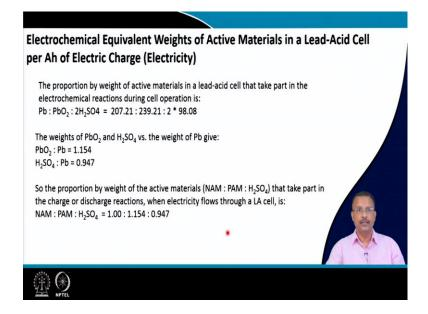
So, the in proportion by weight the active material in lead acid cell take part in this electrochemical reactions. So, lead is to lead oxide is to twice H 2 SO 4 that is coming around these values. So, weight of lead oxide and H 2 SO 4 versus weight of the lead that gives lead oxide is to lead is 1.154 from the calculation and H 2 SO 4 is to lead is 0.947.
