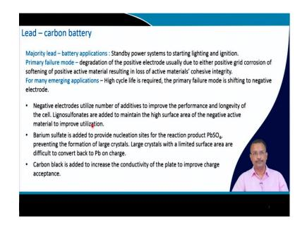
So, the major applications of lead acid battery is the standby power system and particularly this starting lighting and ignition that is used we call it SLI. So, this for the car system that lead acid still today it is using quite heavily and for standby power system for the UPS there are also lead acid batteries being used quite extensively till today.
