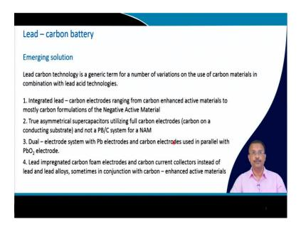
So, lead carbon technology that is basically an emerging I mean a generic term and this is one of the emerging solution for a number of variations on use of carbon material in combination with the lead acid technology. So, you are using this carbon material with this lead acid technology which is about 150 years old technology. So, there are different part I mean various way you can do that; the 1st one is integrated lead carbon electrode that range carbon enhanced active materials.
