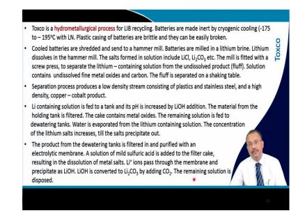
Now, Toxco this is having a hydrometallurgical process for lithium ion battery recycling. So, batteries are made inert by cryogenic cooling, so minus 175 to 195 degree Celsius with liquid nitrogen. So, that is inert battery you can make by such a low temperature and plastic casing of the batteries are brittle and they can easily be broken.
