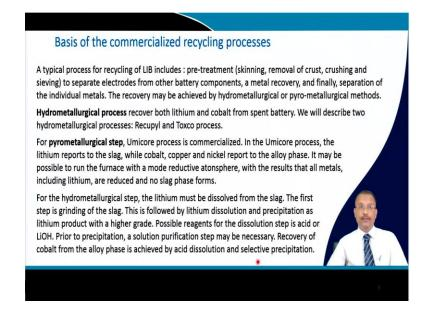
Typical process of recycling of lithium ion batteries that basically includes the pre treatment where is included the skinning and removal of crust then crush and sieve to separate the electrode from other battery component, then a metal recovery and finally the separation of individual metals.
