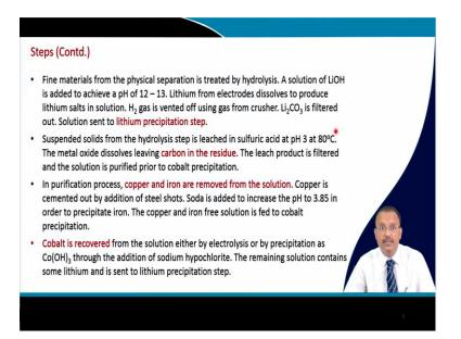
Now, fine materials that you get from the physical separation that is treated by hydrolysis and in this hydrolysis process a solution of lithium hydroxide is added to achieve a pH about 12 to 13. And lithium from the electrodes they dissolve to produce lithium salts in the solution.
