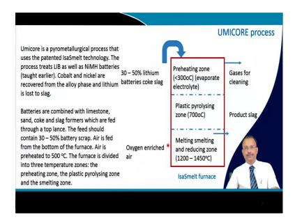
Umicore process that is a pyro metallurgical process it use a patented isasmelt technology and this process treat lithium ion battery as well as nickel metal hydride batteries which I think I have mentioned earlier. Cobalt and nickel are recovered from the alloy phase and lithium is lost to the slag.
