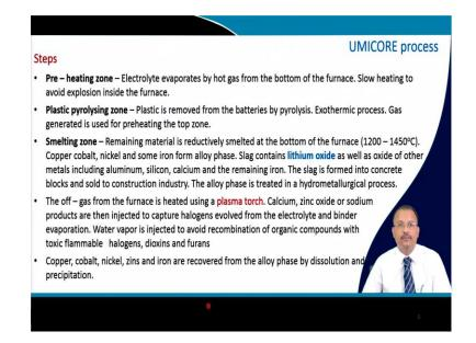
Now, in the preheating zone electrolyte evaporates by hot gas from the bottom of the furnace and usually slow heating is done to avoid the explosion inside the furnace. Then you have a plastic pyrolysing zone and plastic is removed from the battery by pyrolysis its exothermic process.
