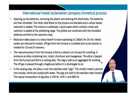
Then finally, the US based company Inmetco International metal reclamation company, so the steps are as follows first the opening of the batteries removing the plastic and draining the electrolyte that is we will have to be done manually. Leave apart the whole battery pack extraction, so that will have to do the do actually manually because there is no automated process because of the shape of the battery already I described it in my earlier lecture.
