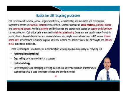
So, as you know the cell is composed of cathode, anode, organic electrolyte, separator those are laminated and compressed together to create electrical contact between them. So, cathode is basically made of active material, then you have polymer binders and conducting carbons. Anode is graphite and both anode and cathode are coated on copper and your aluminium current collector according to the current technology whatever cells you are having.
