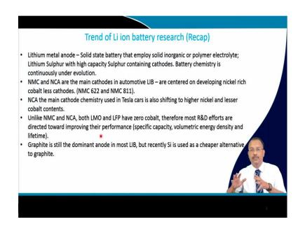
So, let us have a look of the trend of lithium ion battery research and this is mostly a recap already we have talked about it. Lithium metal anodes it is solid state battery that employ solid inorganic or polymer electrolyte. So, lithium metal anode that is in lithium polymer batteries that is one they directly use the lithium metal foils.
