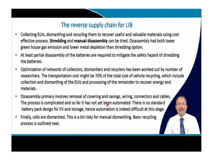
So, collecting ELV, dismantling and recycling them to recover useful and valuable material using a cost effective process that is the thrust of this kind of recycling. So, shredding can be done and manual disassembly these two things can be tried. So, if you disassemble it is having a lower green house gas emission and lower metal depletion than the shredding operation. So, but this is manually you will have to do.
