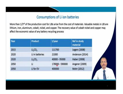
The consumption of lithium ion batteries you can see more one - third of the production cost of lithium ion batteries that arise from the cost of the material, so 33 percent around. Valuable metal in lithium ion batteries there are lithium, iron, aluminium, cobalt, nickel and copper you know, where from they are coming right.
