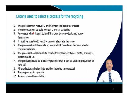
There are certain criteria that you must follow to select a process for recycling the first one is the process must recover lithium and cobalt from the battery is treated. So, some of the company they use only lithium extraction the Belgium base Umicore, but cobalt also it is mandatory. So, that also needs to be extracted recovered. The process must be able to treat lithium ion car batteries. So, not only cells, but from the battery itself the battery module as a whole should be recycled.
