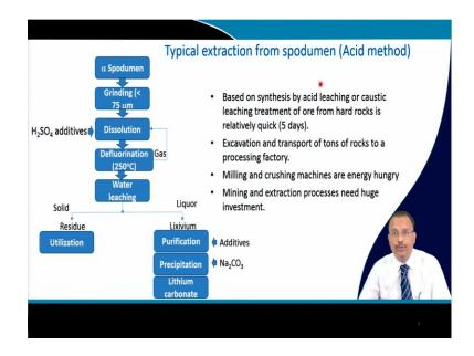
So, there are acid method and base method of a typical extraction of the spodumen and roughly I have summarized that how they are extracted. So, alpha spodumen is used and then it is a very hard rock. So, you will have to grind it to a typical size about 75 micron by using the brushing units.
