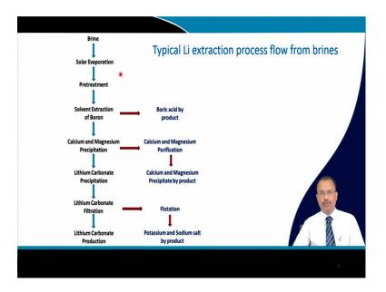
So, the typical extraction from the concentrated lithium containing brines is from the brine you have solar evaporation, then certain kind of pretreatment is there, then solvent extraction of boron and then you get boric acid by product, then calcium and magnesium precipitation takes place and calcium and magnesium they are purified. So, this brines are rich in mineral resources. So, you get other material as well.
