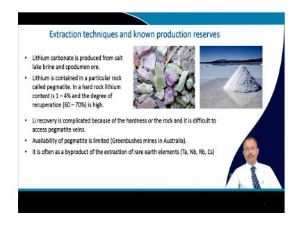
Lithium carbonate is basically produced from salt lake brines and spodumen ore and the spodumen ores basically looks like this. And if you see the brine it is just like salt extraction. So, these are the salt lake brines and you can extract lithium by suitable chemical processing from this brines. So, this is a particular rock that is there in the spodumen ore and that is called pegmatite.
