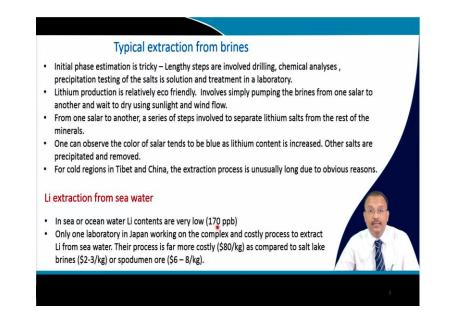
So, in this cases from brine extraction the initial phase of estimation exactly how much lithium content is there. So, that is quite tricky and it is a lengthy step and it involve drilling and then followed by chemical analysis and followed by the precipitation testing of the salt in solution. So, that is usually done in a laboratory. So, that is a lengthy process. It cannot be over by 5 days as we have seen in case of ore extraction of lithium.
