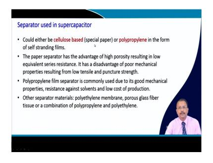
So, these are the primary requirement and usually, the cellulose base is a special paper some of one of the schematic, I showed that the paper separator is used or polypropylene, that is in the form of a self stranding films that is used. Paper separator, they are high porosity and therefore, low ESR value is obtained on the paper separator. But it has poor mechanical properties as you can understand.
