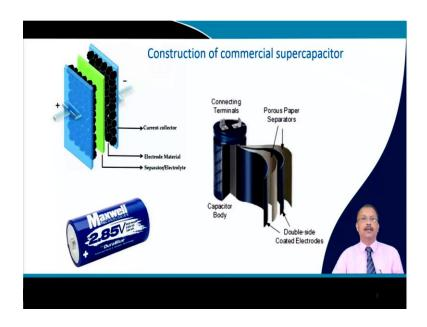
So, if you see the construction, this is the basic construction. So, you should have a current collector and then, you have a coating of either EDLC or a pseudo capacitative material and then, you have a basically a separator which is soaked in electrolyte. And then, you have another electrode and then, you have some kind of contact made so that it is connected to the external circuitry.
