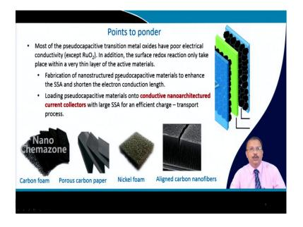
So, in case of a super capacitor, mostly pseudo capacitive transition metal oxide that is used and as I have told you that they have poor electrical conductivity except RuO 2, they are metal like conductivity. So, the surface redox reaction only take place within a very small thin layer. So, therefore, this layer is pretty thin.
