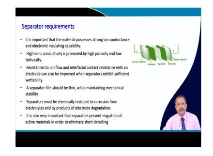
The separator is something similar. The use of it is something similar to that what we described in case of a battery. So, it should have a electronically insulating capability. So, the positive and negative electrodes should not touch and ion should pass through it and therefore, it should be porous in nature and resistance to ion flow and interfacial contact resistance with an electrode that also be improved when super separators, they exhibit sufficient wettability.
