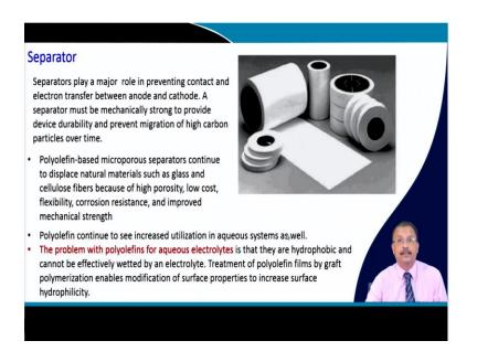
So, as I said that it prevents direct contact and electron transfer between the positive and negative electrode. It should be mechanically strong and durable. So, polyolefin based microporous separator. They are actually replacing this glass and cellulose fiber kind of things because of their porosity and cost of production is also quite low, they are flexible and for the flexible power I mean super capacitor they are quite adaptive for industrial use.
