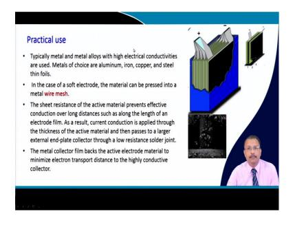
But in practical case, this is not industrially viable to make this kind of structure for bigger capacitors. So, usually, metal and metal alloys which are having reasonably high electrical conductivity that is used. So, this is a type of orientation that is done so that you have a parallel connected capacitors.
