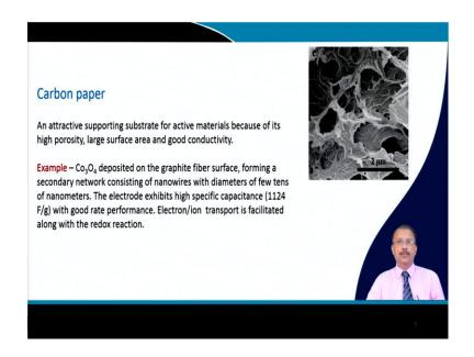
So, if you consider this carbon paper, so that is a supportive substance for the active material. So, it has very high porosity and surface area is also large, conductivity is good. So, one example is that a graphite fiber surface, then this pseudo capacitor that is decide I mean deposited. So, it forms basically a secondary network that consist of the nanowires of this material with a few 10s of nanometer.
