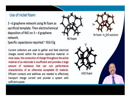
So, carbon paper is considered one of this electrolyte and nickel foam that is also used. So, this is a typical structure one can make. So, this is a foam made out of nickel. And this is basically a sacrifice template and then, electrochemically deposit nickel oxide on a 3 - d graphene network. This is also important to increase this specific capacitance.
