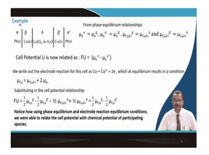
I will cite one example. So, this is the chain platinum – one metal, then copper, then copper sulfate in  $H_2O$ , then you have another copper metal, and then you have a current collector. So, from our definition, phase equilibrium relationship this equation is valid.
