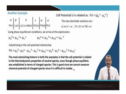
I have given here another example, the same kind of electronic chain. And I leave it on you to calculate this value, the electron chemical potential in alpha and electron chemical potential in alpha dash. Now, here you must remember that it is not a single phase relation here I have put lithium. So, lithium is getting oxidized and you have also titanium chloride salt here.
