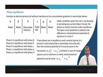
Now, we will talk about the phase that is there inside the material. So, you can see in an electrochemical chain you have metal which is current collector. Then you may have another metal like copper, then you have electrolyte solution. Then you have inside the electrolyte solution a solid salt. Then you have another metal and then you have the final current collector.
