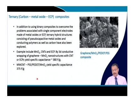
Then you can have the third category, a ternary kind of system which uses carbon, and then metal oxide and electronically conducting polymer composites So, this is one example. Graphene is a carbonaceous material; M n O 2 is a pseudo capacitive, and PEDOT PSS that is the polymer part. So, this is a hybrid structure and also sometimes manganese dioxide CNT and ECP is used.
