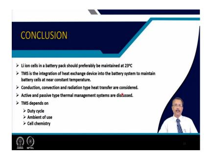
So, in this particular lecture we talked about lithium-ion cells in a battery pack should preferably be maintained at a temperature around room temperature 23 degree Celsius. Thermal management system is the integration of heat exchange device into the battery system to maintain battery cells at near constant temperature.
