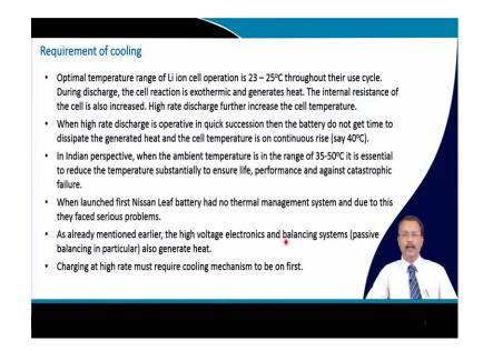
Not always heating is required, sometimes cooling is also required. So, if I consider that optimal range is in between 23 to 25 degree Celsius the normal room temperature throughout the their cycle, then it is ok. During discharge the cell reaction is exothermic and it will generate heat. The internal resistance of the cell also will increase the high rate of discharge further increase the cell temperature. So, this will be deviated from this right.
