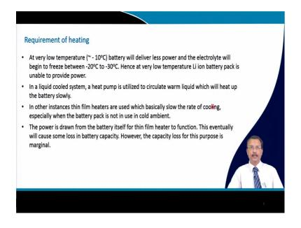
Now, not always as I said that cooling is required. Sometimes, you need to heat the battery also. For example, at very low temperature say minus 10 degree Celsius, the battery will deliver less power and the electrolyte will begin to freeze at typical temperature. You remember in the electrolyte we have a lithium-based salt and a cyclic and a linear types of mixture solvent.
