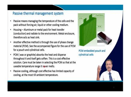
Now, this all are part of active thermal management system. You can have a passive thermal management system where automatically it gets cooled not really automatically. So, passive means the managing the temperature of the cells and the pack without forcing any air or liquid or other cooling medium.
