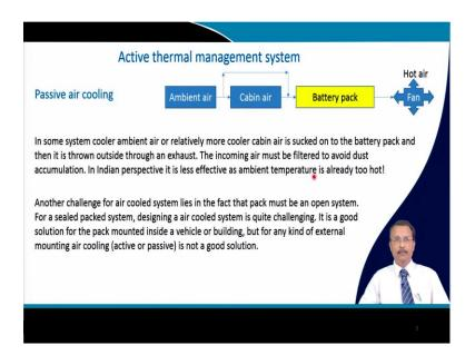
Passive air cooling that is also quite interesting. You have the ambient air here, it is not very effective in our perspective. So, unless you are using a air conditioned car. So, this air is sucked and that partially cool the battery pack and the hot air is discharged in the ambient. So, in some particular system cooler ambient air or relatively more cooler cabin air that is sucked to the battery pack as I mentioned and then thrown outside through a some kind of exhaust.
