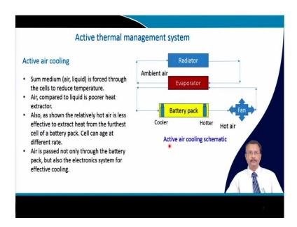
So, active thermal management system is a active air cooling. So, sum medium air or liquid that is forced through the cell to reduce the temperature. And this is a schematic of active air cooling system. So, here you can see that you have a radiator here. So, ambient
