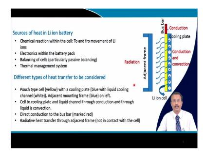
So, what are the sources of heat in lithium battery? Almost it is unavoidable. And this is due to the chemical reaction within the cell. And lithium is going to fro from cathode to anode during charging and during discharge from the negative electrode to positive electrode. So, it generates heat. You are using lot of electronics. You know that in the last lecture, we talk about the master control board, then the slave boards and lot of electronics are involved and they also dissipate heats.
