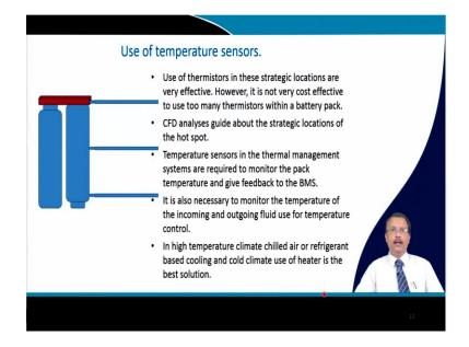
Now, where should we put this kind of temperature sensor? So, use of thermistor in these strategic locations are very effective. So, either you can put it in the bus bar of course, you cannot put it inside the cell. So, you will have to put it at the surface of the cell. So, in the bus bar is one location where the temperature should be monitored, second location is here as you can see, and third one is just at the middle of the series connected pack.
