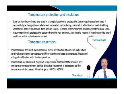
Temperature protection and insulation is also required. So, steel and aluminum sheets that are used as a strategic location to protect the battery against the radiant heat. A sandwich type design two metal sheets separated by insulating material is quite effective for the heat shielding. Same like your furnace construction you have metal sheet and you have refractory therein.
