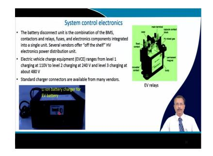
So, this battery disconnect unit is basically a combination of BMS then contactors and relays, fuses, electronic components integrated into a single unit. And several vendors they offer the "off shelf" so, HV electronics power distribution board. So, you can purchase it.
