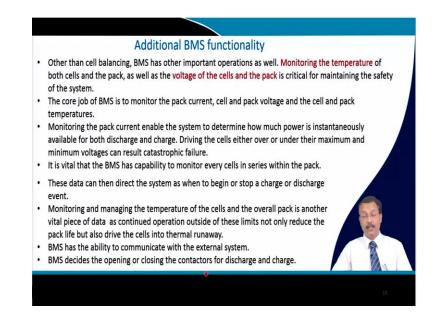
So, apart from this balancing there are additional BMS functionalities. So, they have one important operations that one can mention is monitoring the temperature of both the cells and the pack, together with that they monitor the voltage of the cells and the pack and these two are critical for maintaining the safety of the system, it may not be over charged temperature should not rise beyond a certain limit.
