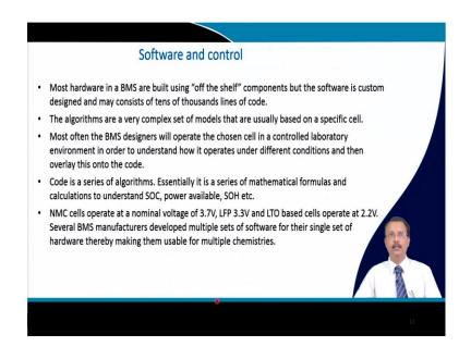
Software part is very important most of the hardware you know that although the design part is important for the PCB, for the controller, for the slave boards ASIC is already "off the shelf" one can purchase, most of the component in fact, one can purchase off the shelf, but the software is custom designed and may consist of thousands lines of code. So, that is another area which is important and we also take help of other scientists in this area to write this codes.
