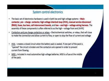
Now, while you design this BMS there are many system control electronics that is important. So, each of them has have their particular functions and I am not going into the details, but you should know exactly that what are the components that is used.
