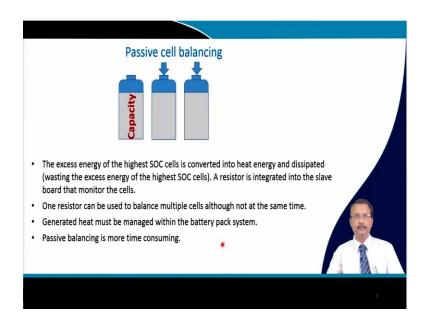
So, first we will talk about the passive cell balancing and this is quite straightforward, the excess energy of the highest SOC cell. So, this one was the highest and this one also was the highest. In fact, these two cell capacity was higher as compared to this one this is converted into heat energy and dissipated.
