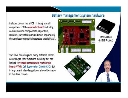
So, this photographs they were taken from our own work because we are also in a process as a part of my sponsored project we are making a 28 volt 16 ampere hour lithium ion battery pack for certain specific use and this is one typical PCB that you can see. So, this is the type of control board how it looks like. So, it basically integrates all components that is there in the controller board.
