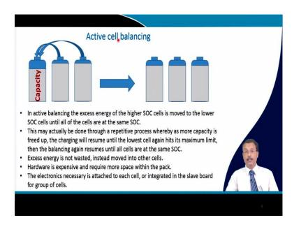
Second one which is although expensive and little bit more design aspects are required to do that is the active cell balancing for our case we are in the process of doing it, but this is done this is usually done for a good battery pack. And the active cell balancing the excess energy of the higher state of charge cells is move to the lower state of charge.
